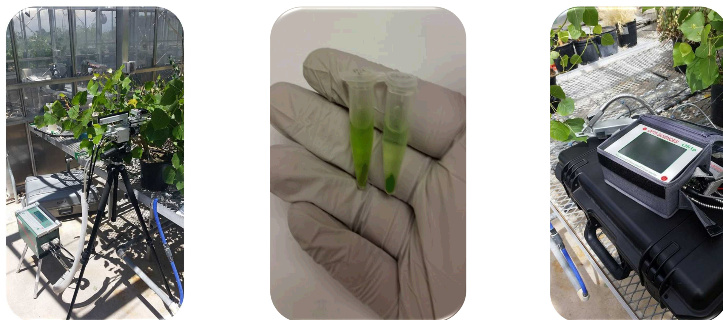
Figure 2. a.) Gas exchange data are collected in the rooftop greenhouse. b.) Chlorophyll extracts. c.) Effective quantum yield data is collected in the light then the leaves are dark adapted before optimal yield is taken.
