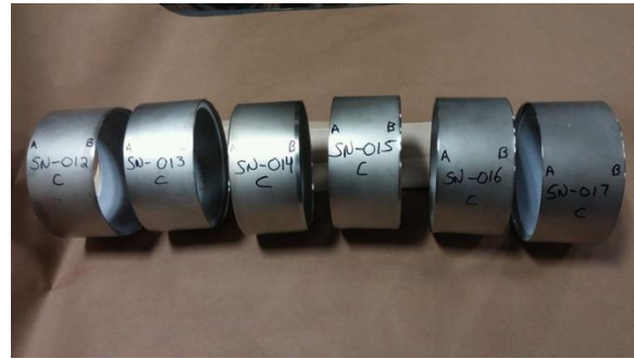
Figure 6. (a) compression ring assembled with fixture. (b) ring assemblies s/n 012-017
