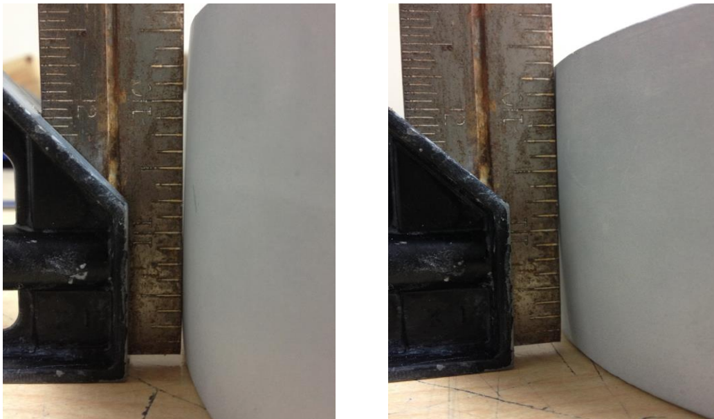
Figure 2. Distortions in the OD of the rings that were cast
