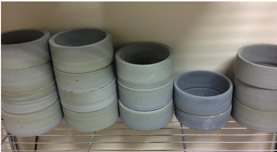
Figure 3 Lossy ceramic rings prior to final grinding of the outside diameter.
