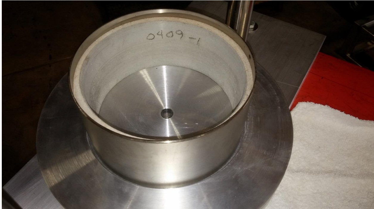
Figure 10: Shown is a toroid compressively inserted into a steel sleeve.
