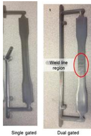
Figure 20. Picture of single gated and dual gated test specimens.
