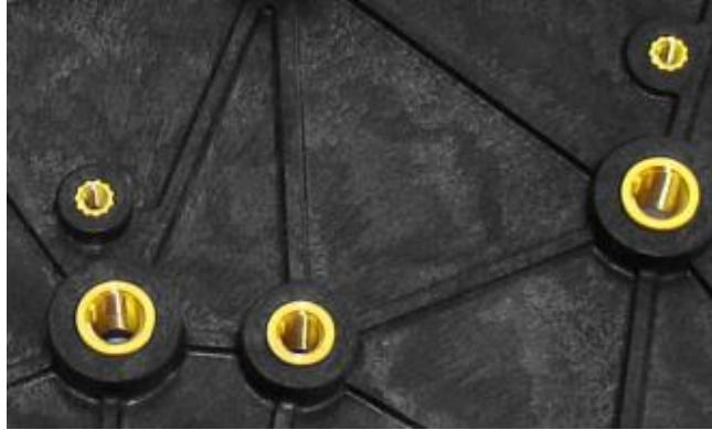
Figure 71. A molded part by an insert injection molding [137]
