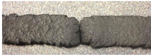
Figure 74. Short shot dual gated dog bone specimen depicting accentuated melt freeze-off and weld line
