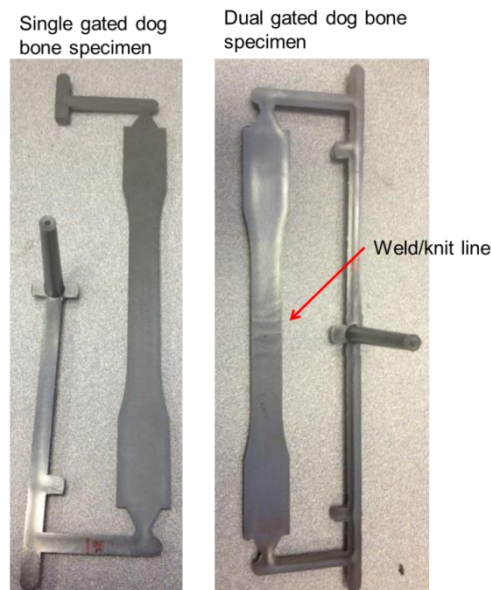
Figure 9: Images of single gated (left) and dual gated (right) injection molded dog bone specimens made by the University of Massachusetts at Lowell.
