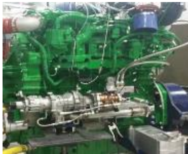
Three Stage Roots Expander on Engine
