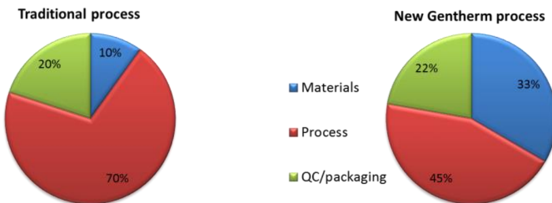
Figure 74 Comparison of manufacturing cost breakdown for traditional TE manufacturing process as compared to new Gentherm process. Significant cost reduction is achieved by reducing material waste and increasing yield through manufacturing net shaped thermoelectric materials.
