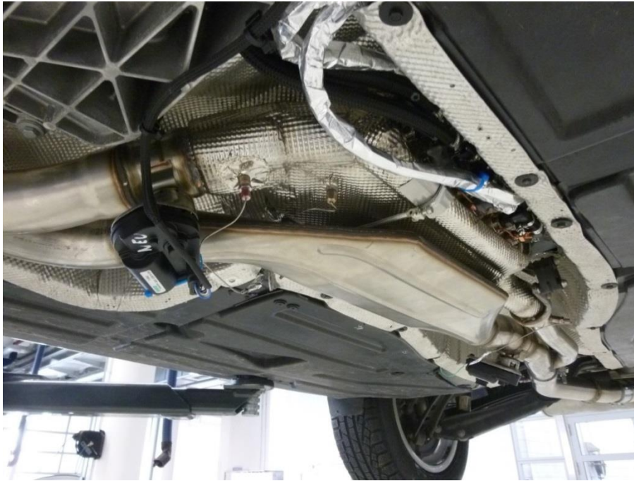
Figure 56 TEG integrated into the exhaust system of the BMW X3 xDrive28i.
