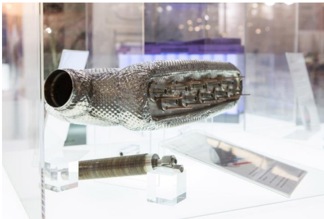
Figure 1 lower left corner: thermoelectric power generation cartridge. Top: passenger vehicle thermoelectric power generation system.
