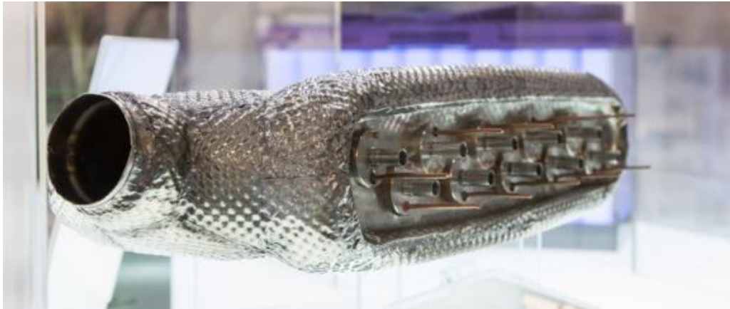
Figure 34 Assembled TEG section of TEG system (canning and cartridges without bypass.
