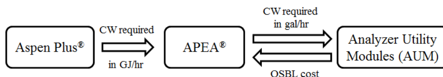
Figure 3-36. Methodology for cooling water system cost estimation using AUM.
