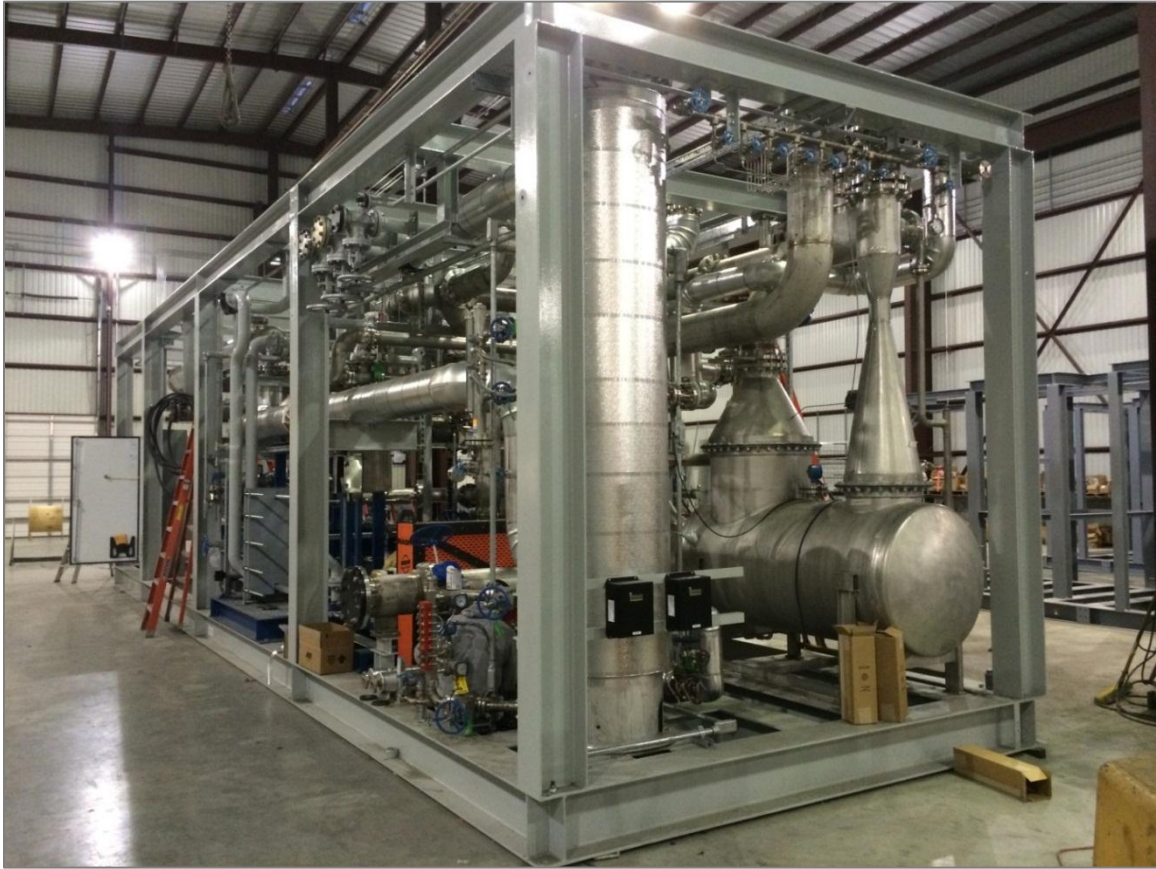
Figure 4.5. Lower level of the 20 TPD system containing rotating equipment and associated vessels during fabrication.
