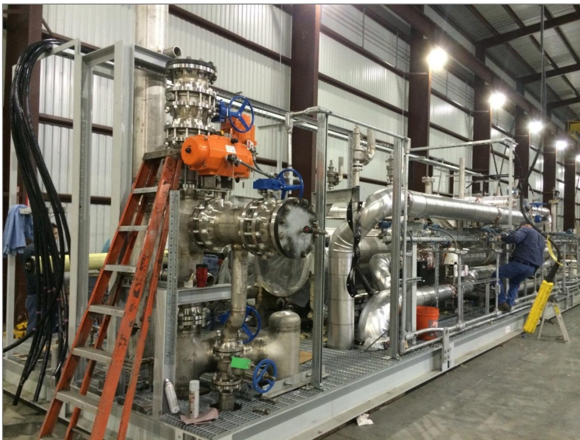
Figure 4.6. Upper level of the 20 TPD system containing membrane module vessels and associated piping during fabrication.
