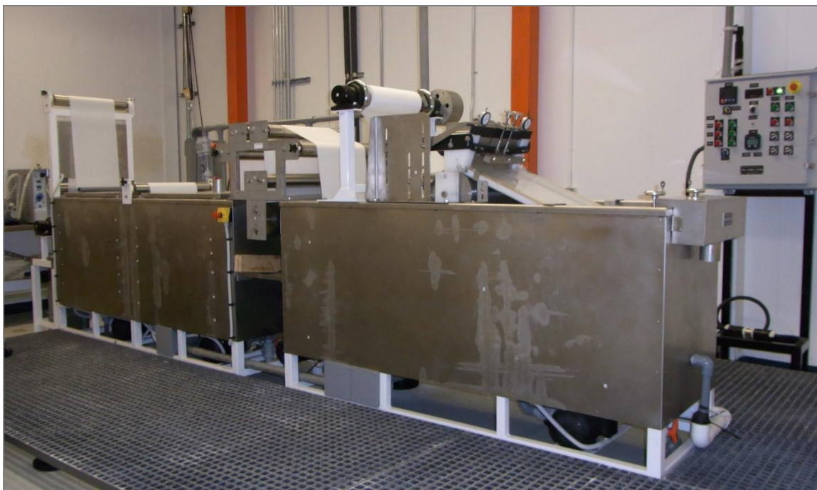
Figure 2.2. A picture of the small casting machine used to optimize substrates for Gen-2 Polaris membranes. The casting tray and quench bath are visible at the center right of the picture. The rinsing/annealing baths and membrane take-up roll are on the left side of the picture.
