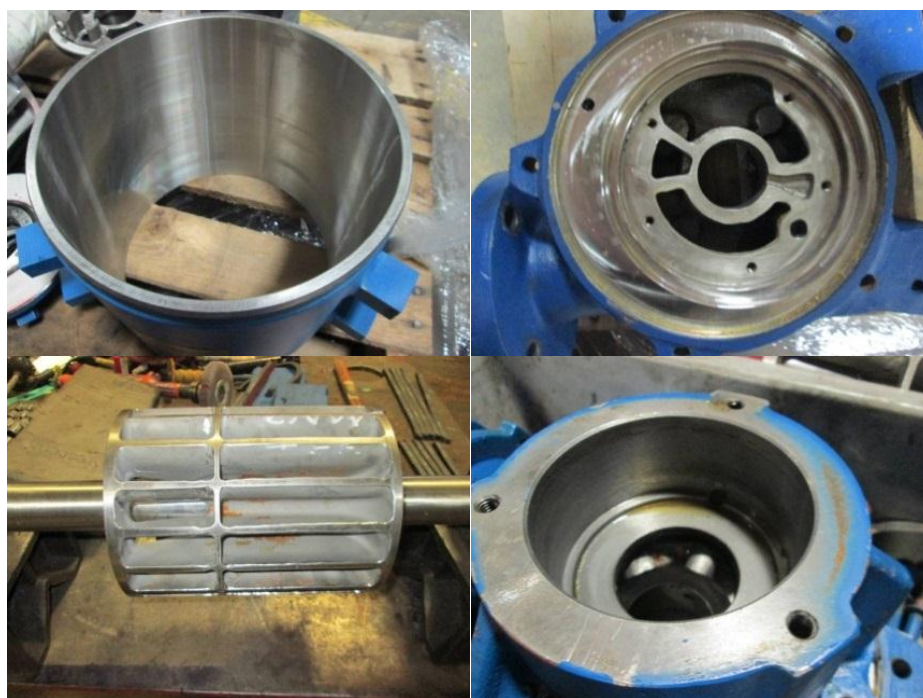
Figure 3.16. Pictures of key compressor components after the liquid ring compressor operated with flue gas for over one month at NCCC in early 2013.
