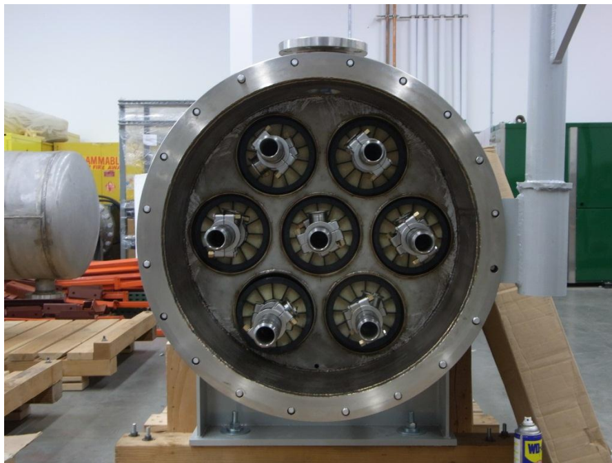
Figure 4.4. Cross-sectional view of a bundled module pressure vessel with spiral-wound modules installed.
