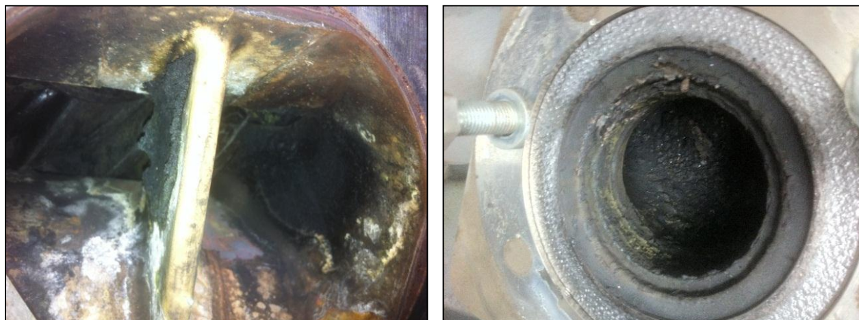
Figure 3.14. Pictures of the feed compressor components showing particulate buildup and corrosion.
