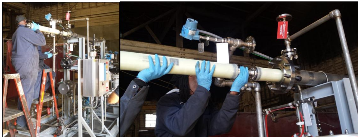
Figure 7.5. Fabricators installing two Polaris 4-inch spiral-wound modules into the Polaris module vessel prior to shipment of the skid in May 2015 at Johansing Iron Works, Oakland, CA.
