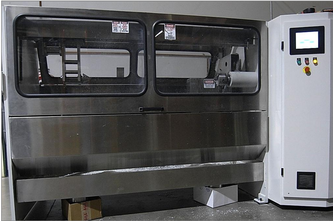
Figure 2.7. Photograph of the membrane module trimming machine designed, commissioned, and tested during budget period 1. The machine allows modules to be fabricated at a faster rate (reduced cost) and with lower pressure drop than the previous technique.
