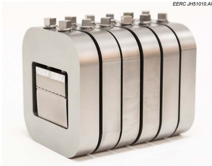
Figure 13. Assembled jig in preparation for heating to bond the APMT plate to the superalloy block.
