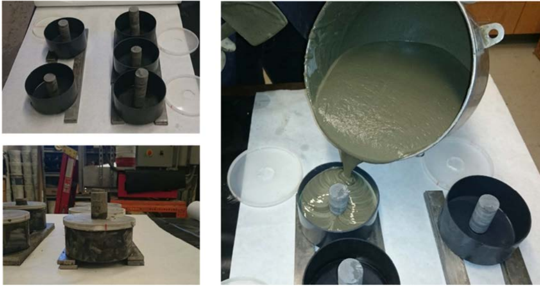
Fig.2.13: Preparation of reference push-out specimen (without repair material).
