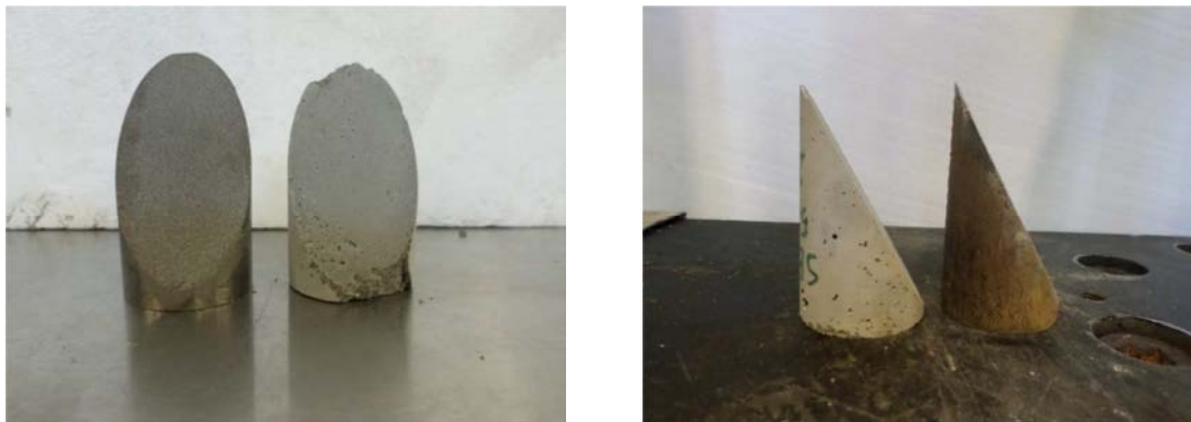
Fig. 2.25: Example failure cones of the slant shear test.
