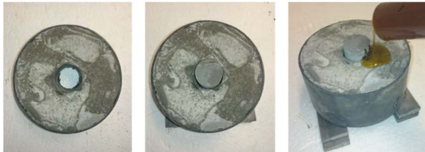
Fig.2.14: Preparation of repaired push-out test specimen with Novolac epoxy.
