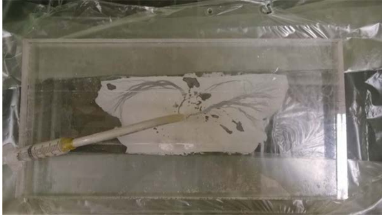
Fig.2.48: Microfine cement injected in 75 microns crack.
