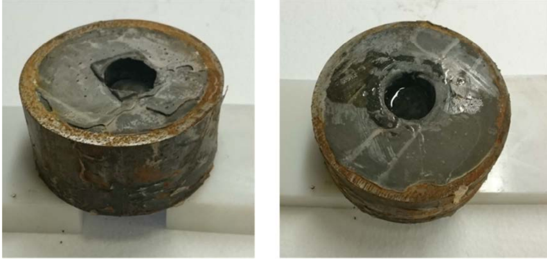
Fig.2.19: Push-out specimens with partial embedment length.
