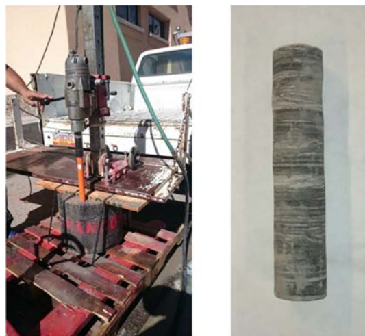
Fig.2.11: Core drilling (left), and obtained shale core (right).
