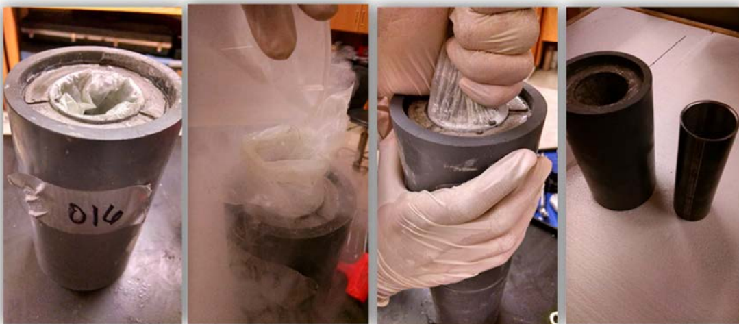
Fig. 3.8 – A sample with a microannulus created by the release film method. From left to right: sample at end of curing showing release film (plastic) on top of sample; cooling casing with liquid nitrogen; removing release film and casing; casing removed from cement sheath.
