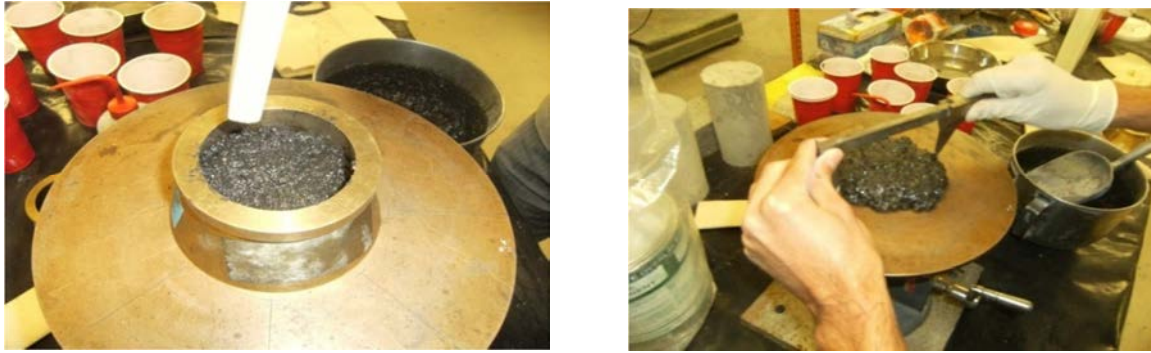
Fig.2.2: Filling the flowability cone (left), and measuring caliper (right).
