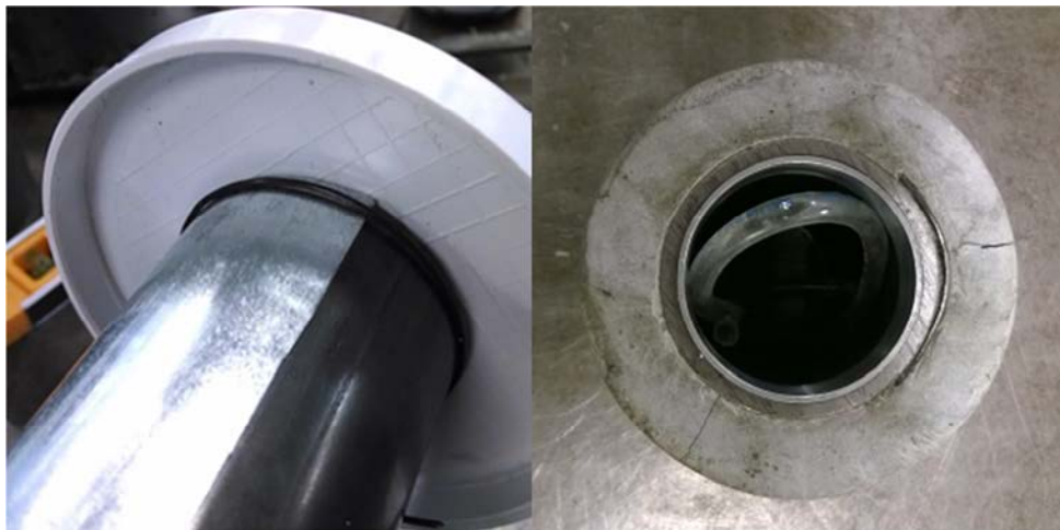
Fig. 3.7: a) Steel sheet attached to the cylinder prior to casting cement annulus to create a 'slot flaw' in the specimen, and b) Cured sample with slot flaw visible at contact between cement and steel casing.
