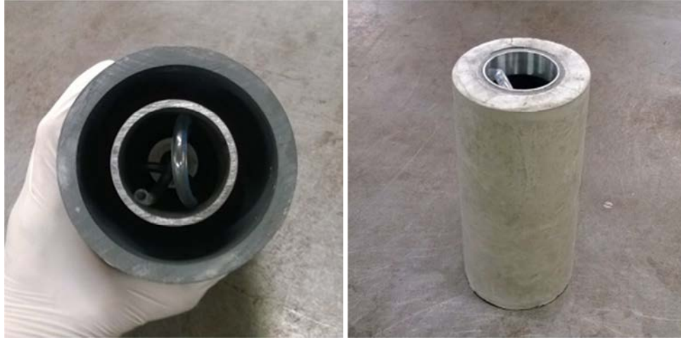
Fig. 3.6: a) Steel centered in mold ready for cement to be poured in annulus. The tube connected to the hole in the steel is visible inside the steel casing. B) Cured sample.
