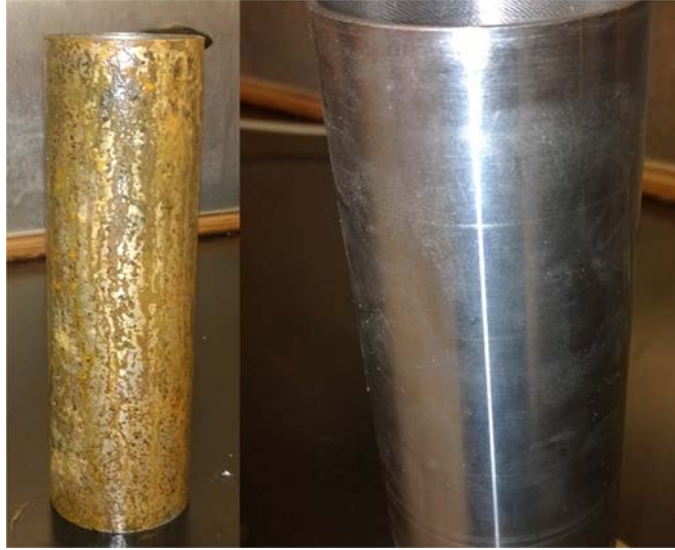
Fig. 3.10 – Casing with (left) and without (right) corrosion.
