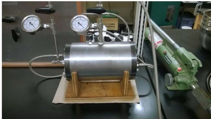
Fig.3.3: Assembled pressure vessel connected to permeameter.
