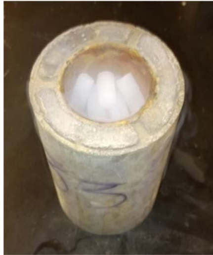
Fig. 3.9: Using dry ice to cool the casing and de-bond the steel casing and cement sheath
