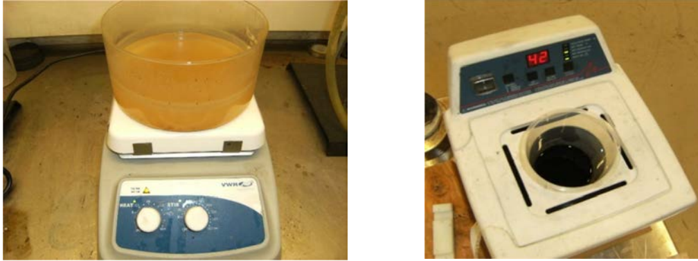
Fig.2.1: Mixing of polymer nanocomposite (left) mechanical stirring (right) sonication.
