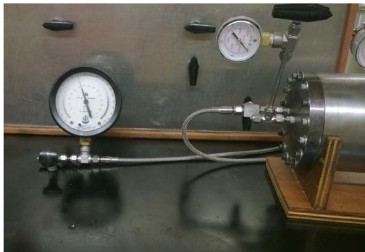
Fig. 3.5: Control valve at downstream to maintain back-pressure
