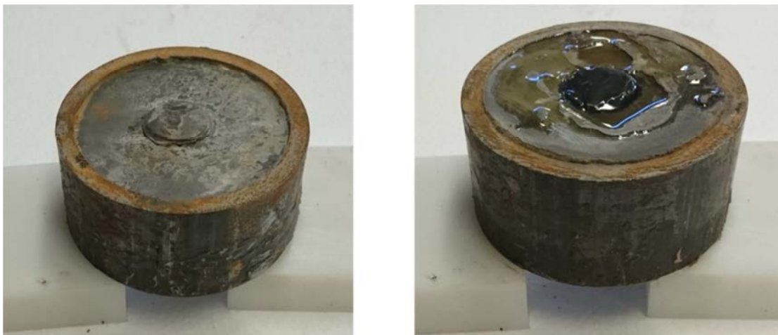
Fig.2.18: Push-out specimens with full embedment length.
