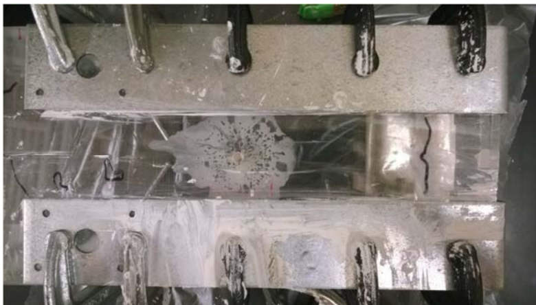
Fig.2.47: Microfine cement injected in 50 microns crack.
