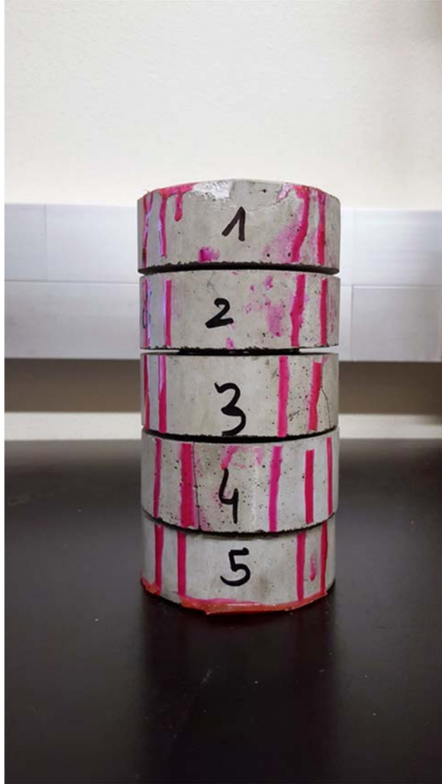
Fig.3.38: Sample 66 after repair with dyed epoxy and sectioning.
