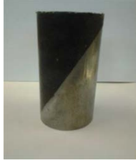
Fig.2.5: Composite cylinder of neat polymer overlay on steel
