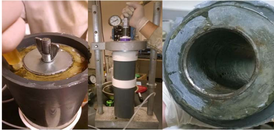
Fig. 3.11 – Figure showing the “epoxy capsule” method for injecting repair material into sample with flaws.
