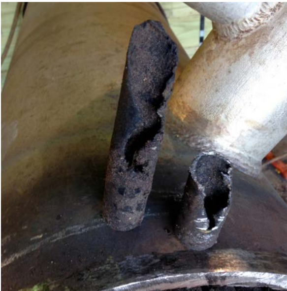
E-120 Tubes after Failure
