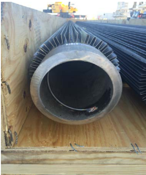
New Heat Exchanger Tube
