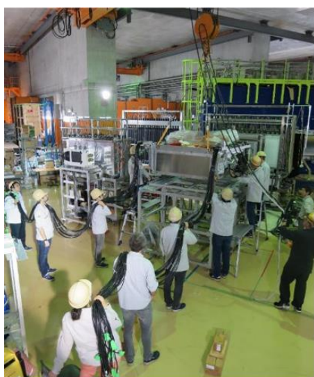
Figure 6: Installation of TPC into SAMURAI magnet
