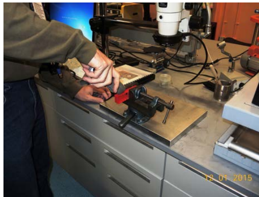
Figure 4. Vice holding jig in place using utility knife to cut
