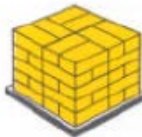
Pinwheel Used where a brick pattern is unstable.
