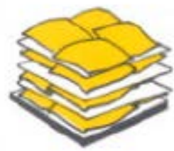
Irregular Stacking Patterns Wood strips, plywood, or heavy cardboard between layers can help stabilize castings, bags, and other irregular shapes.
