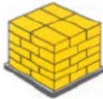
Brick Containers are interlocked by turning each level 90 degrees.
