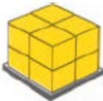
Block The most common. The upper level may require wire or strapping for stability.
