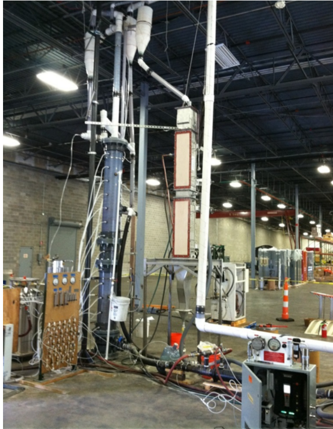
Figure 17. Moving Bed Heat Exchanger Connected to the ADA Cold Flow Model, Modified to Simulate Process Conditions.
