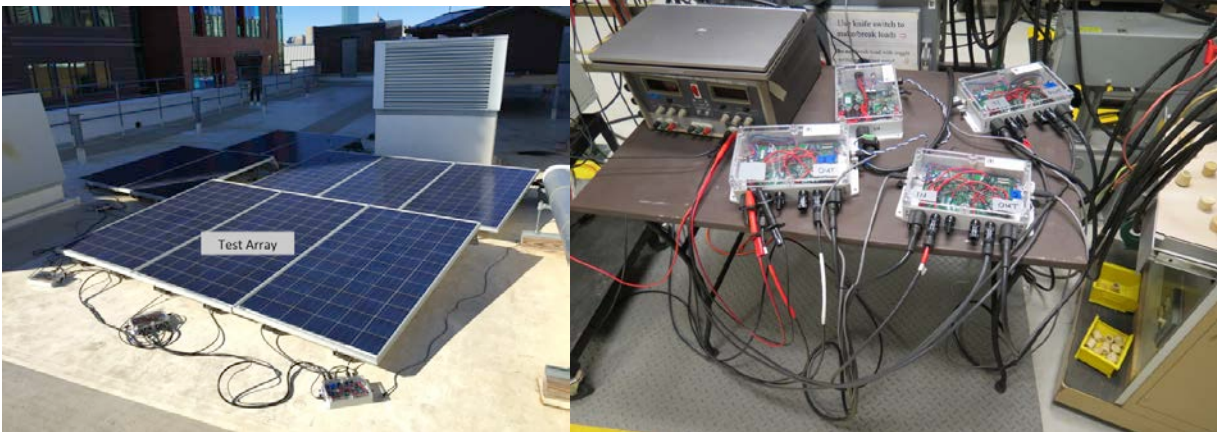
Figure 3-5: Rooftop testing of DE-integrated PV (Left); Benchtop efficiency characterization of DE at Sandia's Distributed Energy Test Laboratory (Right)
