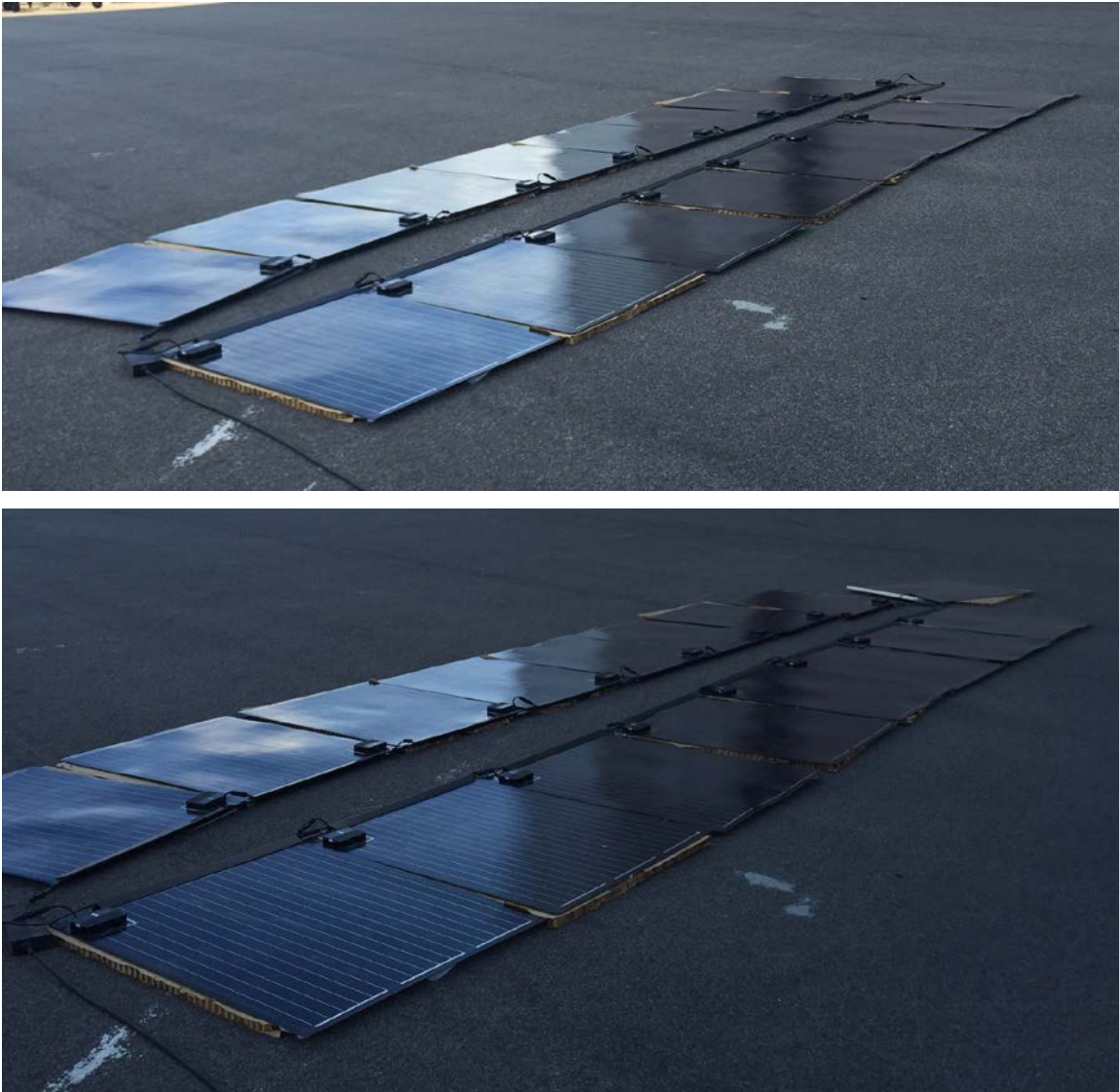
Figure C-1: (Top) “n” module test (proper number of PV modules); (Bottom) “n+1” module test (improper number of PV Modules)
