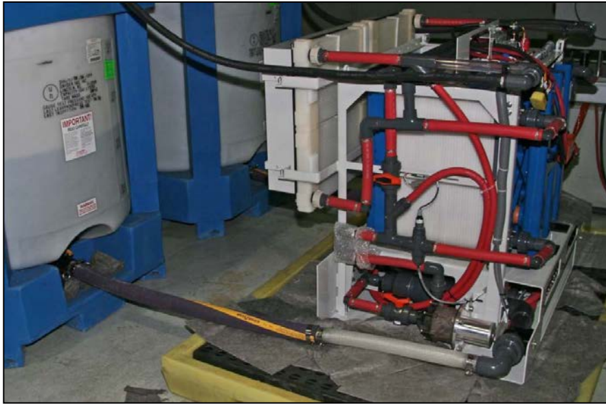
Figure 11. 5kW Prudent Energy Vanadium Redox Flow Battery undergoing testing at ACEP.
