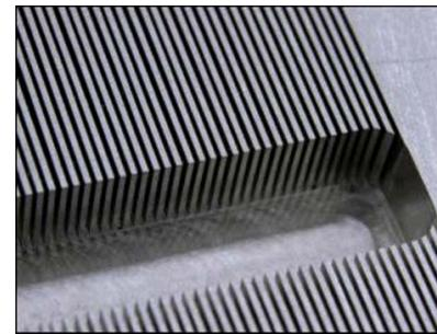
Key element: heat exchange in thin engineered channels
