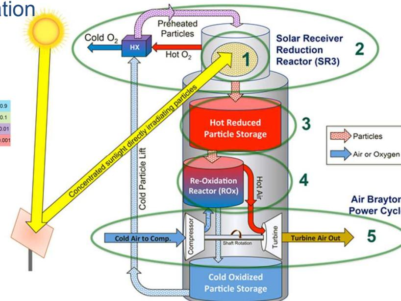
4. Pressurized oxidation reactor. Air acts as reactant and heat transfer fluid. Open cycle – no gas storage.
