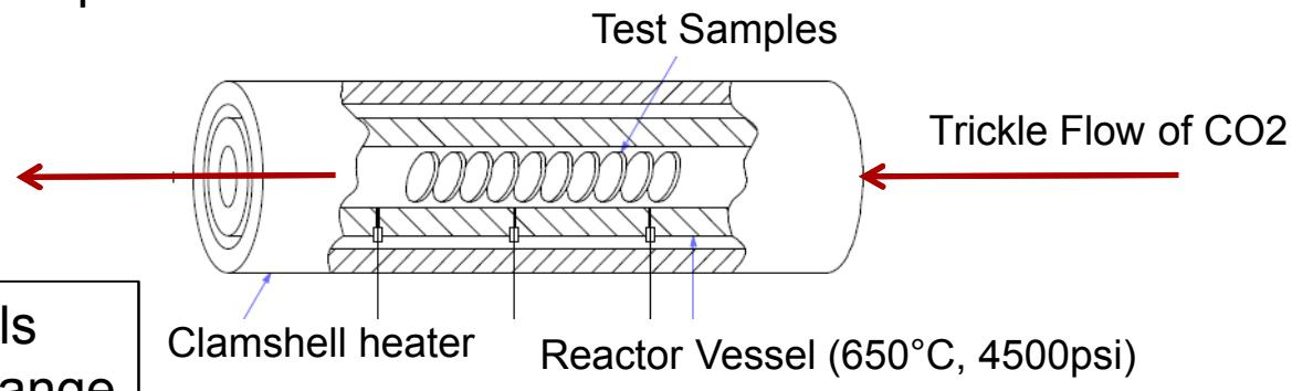
Facility used to test materials performance over operational range of system requirements.
