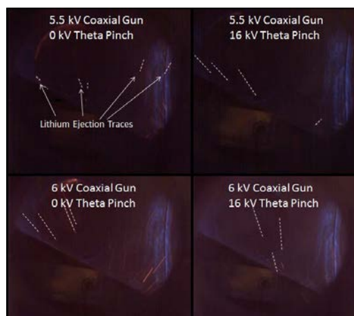
Figure 19. Ejection observed from the 10 and 11 mm trenches as well as the lithium pool in the bottom of the trenches. Increased ejection is observed in the case of the 6 kV coaxial gun shots, however, it is still only observed to be coming from the 10 and 11 mm trenches and the lithium pool.
