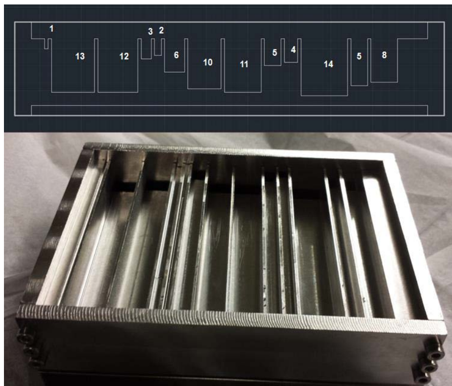
Figure 18. (Top) Schematic of the side view of the special LiMIT channels. Trench width is displayed in millimeters. (Bottom) Photograph of the LiMIT trenches as assembled. Trenches were subsequently installed into the TELS chamber and filled.
