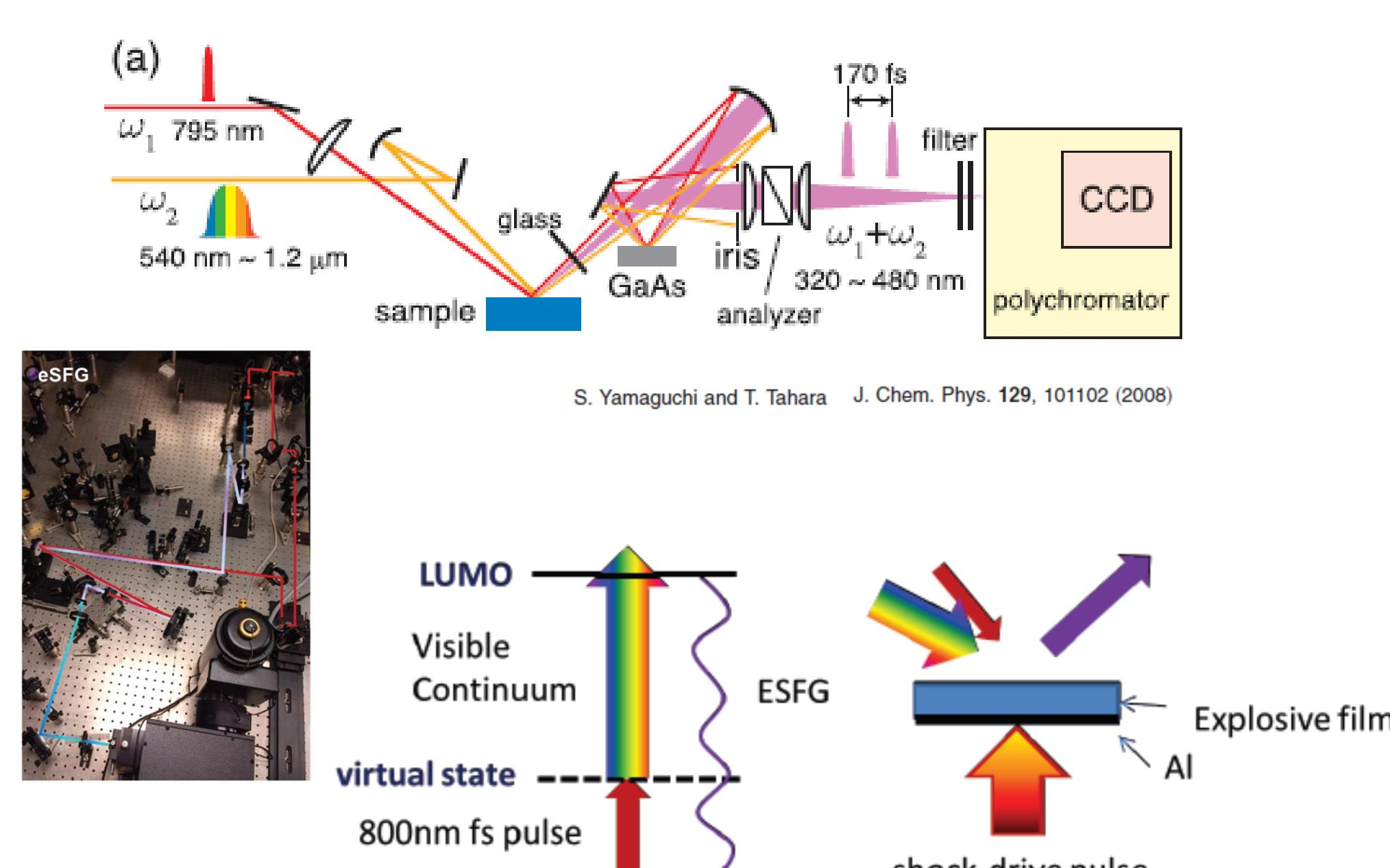
Measurement combines broad-band continuum and narrow-band pulse to generate light at the sum of their frequencies within a few monolayers of the interface. Signal increases when sum matches the HOMO/LUMO gap.
