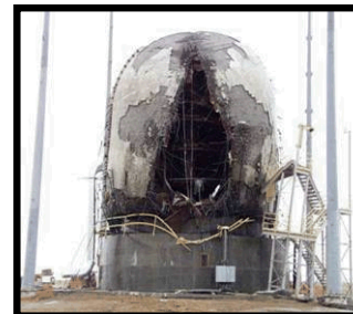
1/4-Scale Prestressed Concrete Containment Vessel Test to Failure (Japan)
