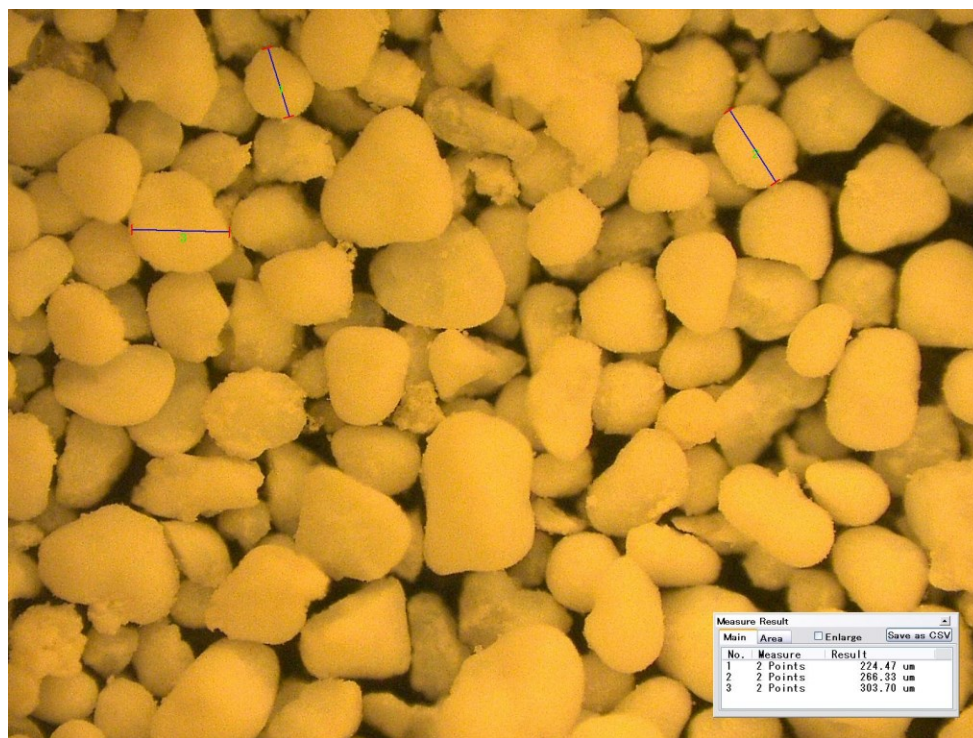
Figure 8. Optical microscope photograph of Mn-imprinted polymer beads.
