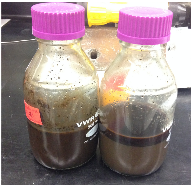
Figure 30. View of products obtained in HTL2 when the solvent in this step was heptane (left), or dodecane (right).
