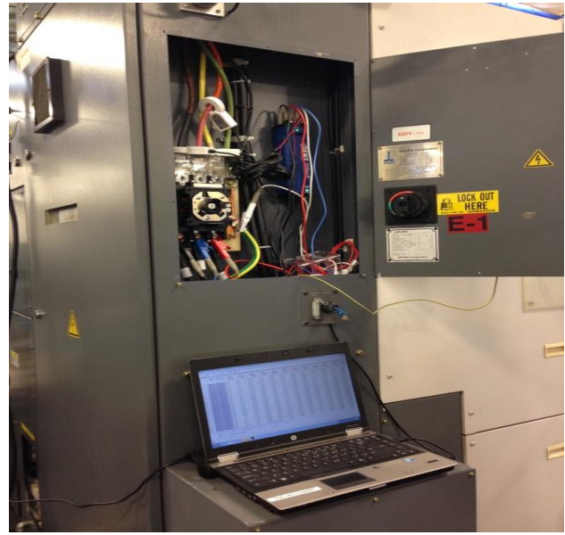
(b) Power meter installed in OKUMA "Twin Star" CNC machine
