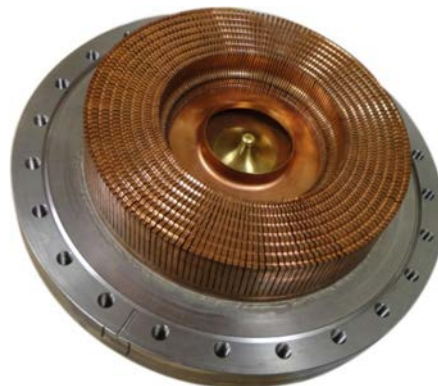
Figure 11: The original CHX, after the fins were manually straightened with pieces of plastic shim to even out the slots.
