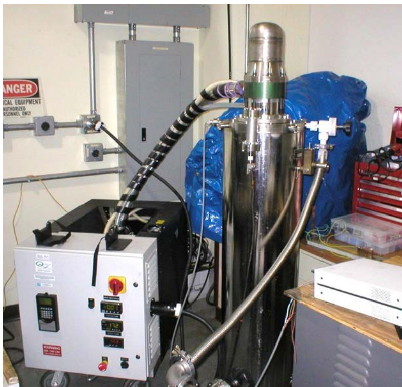
Figure 39: The 2S241K-FAR system developed in Phase II, integrated into a dewar with a test coil at Superpower in Schenectady, NY.
