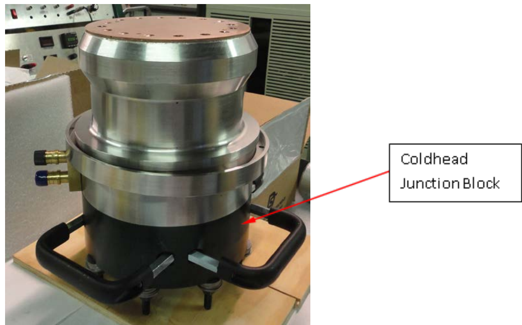
Figure 23: Brazed version of “70K” coldhead going together on the bench.
