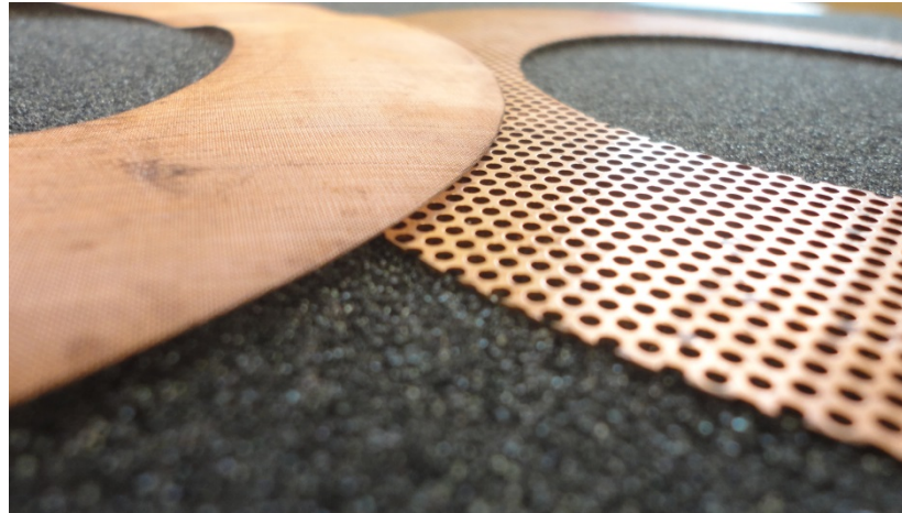
Figure 26: Closeup of fine copper screen (L) vs. perforated ring (R). The ring has much greater thermal mass, but also less open flow area.
