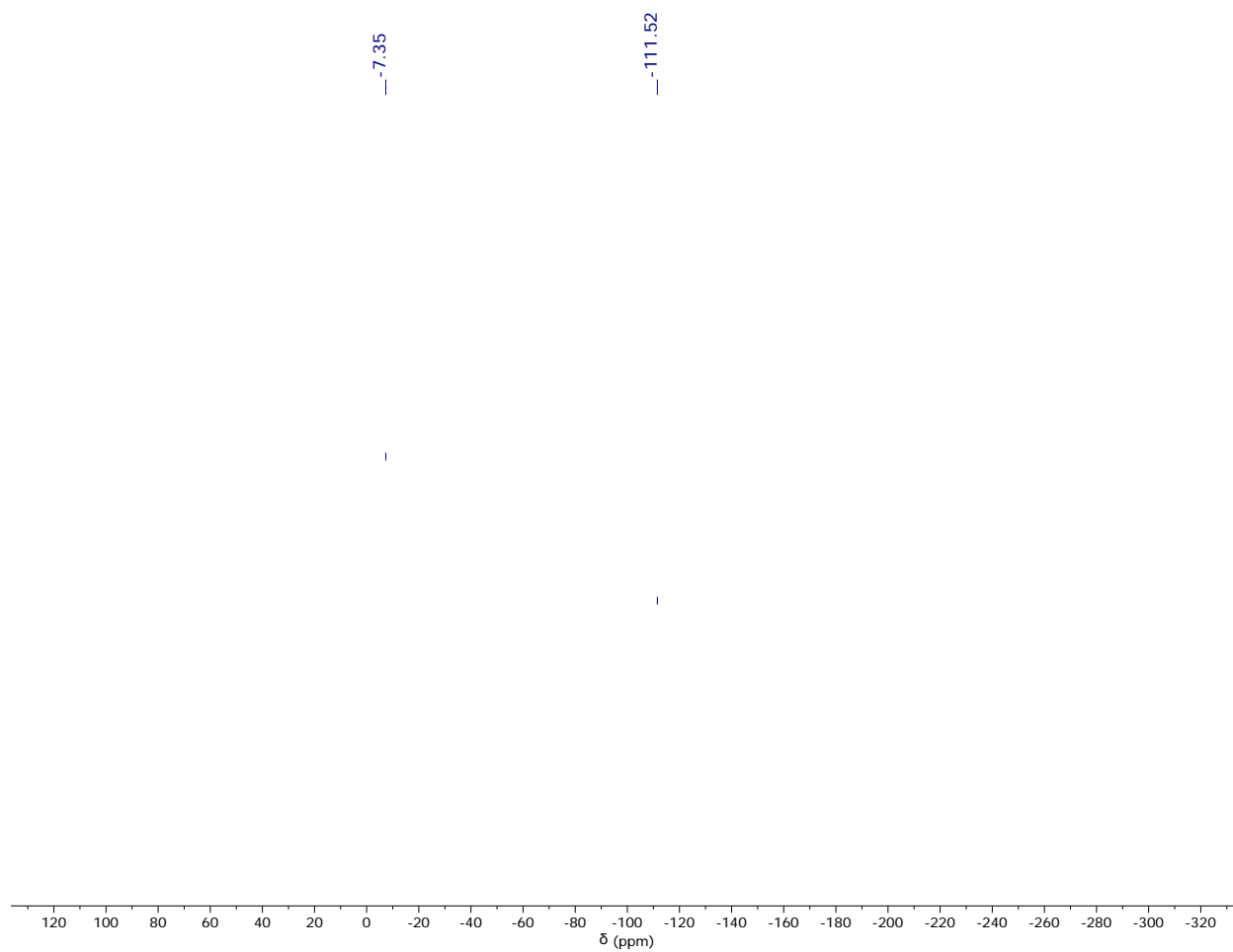
Figure S11. ^{29}\text{Si} NMR spectrum of 3 in \text{THF-}d_8 . The resonance at -111.52 ppm is assignable to the borosilicate glass from the NMR tube.
