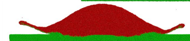
Complex chemical/physical phenomena such as wetting, solidification, and fragmentation captured in atomistic scale modeling.
