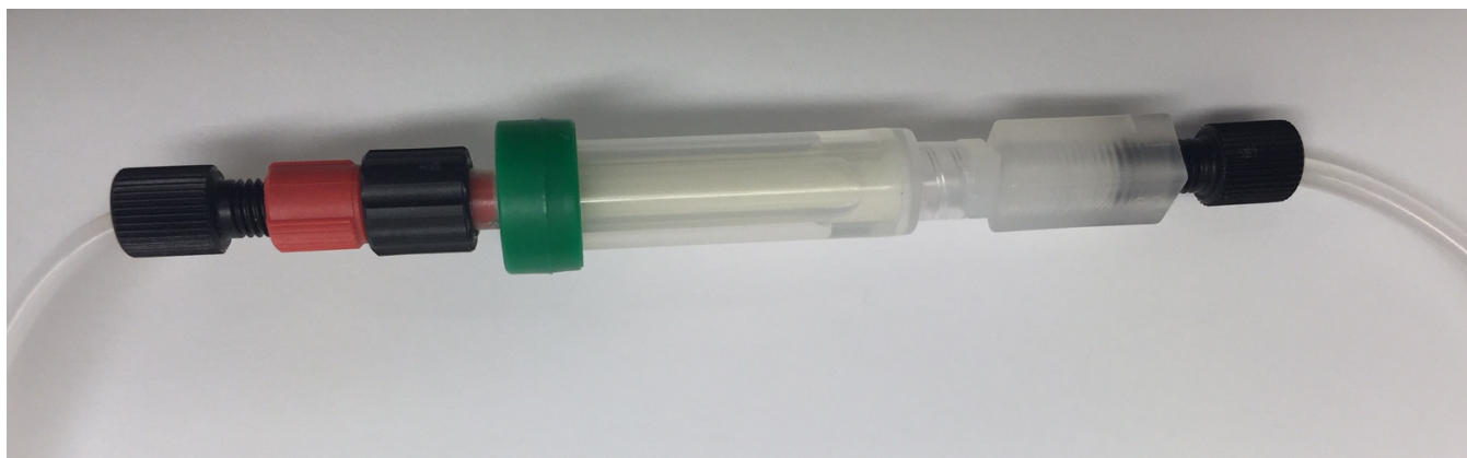
Figure 5: Photograph of Bio-Scale Mini Cartridge (obtained empty from BioRad) filled with mPEG-750 resin.
