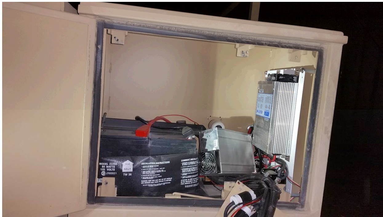
Figure 5: Broken charger behind panel on aerostat trailer
