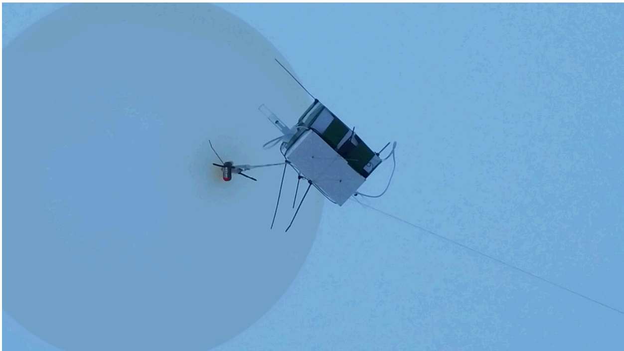
Figure 1: Original side-by-side configuration with 1,600L balloon was unsuccessful
