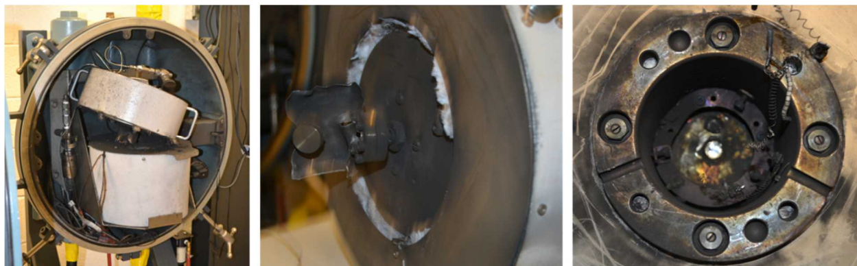
Figure I-3: ARC conditions from attempted evaluation of 18650 cells using NCM523 vs. 10 and 15 wt% nanosilicon.
