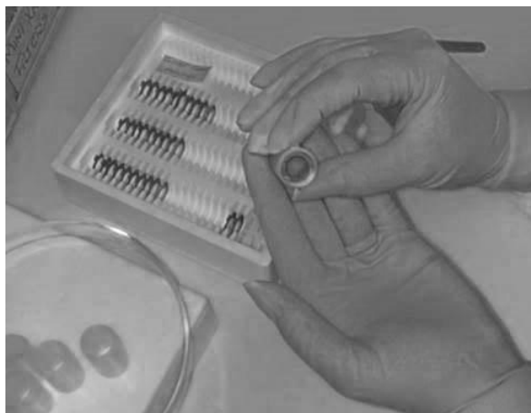
Figure 4. Test fit of filters into tube bodies
