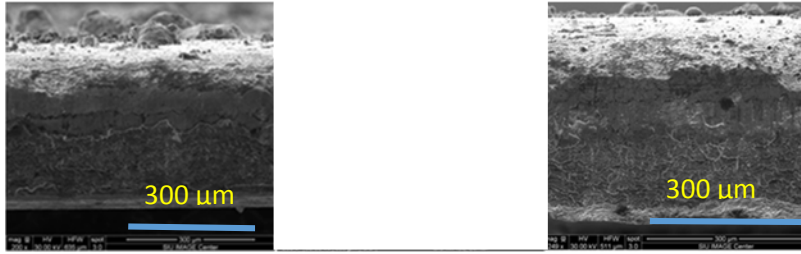
Figure 32. SEM images of the cross section of the two coatings obtained in acetylene and air.
