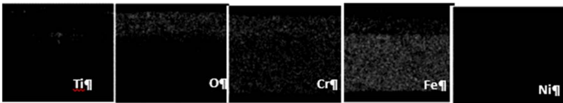
Figure 35. Elemental mapping of the cross section of the as-received sample 11. Coating obtained in acetylene - air flame.
