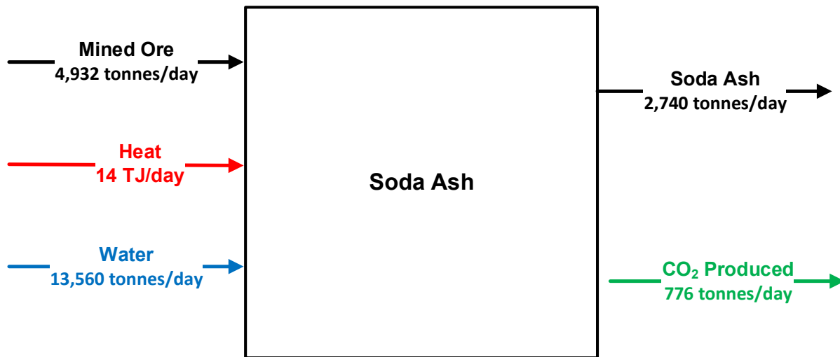
Figure O-1. Material and energy flows for a nominal soda ash (processing from Trona) production plant
