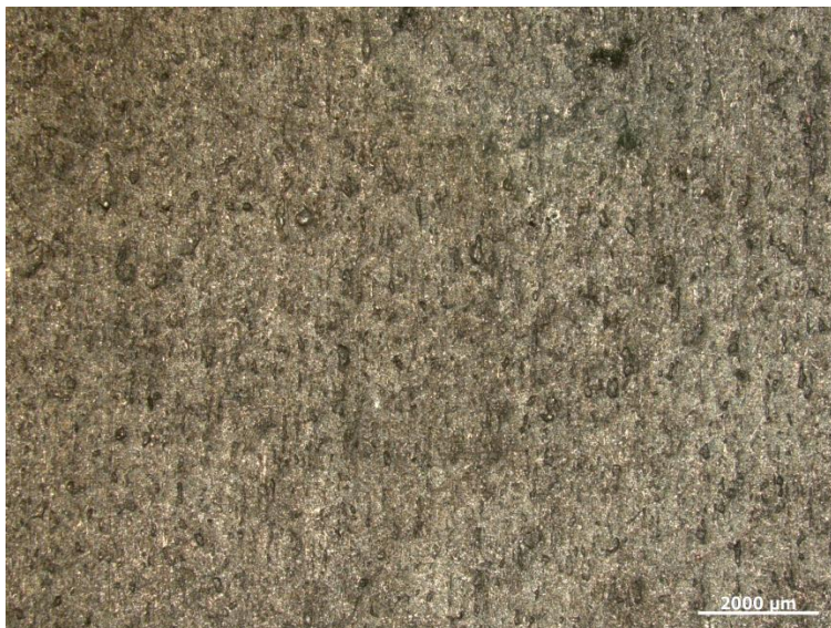
Figure 25. Front and back surface of cold rolled interior slice Zr-clad U-10Mo coupon.
