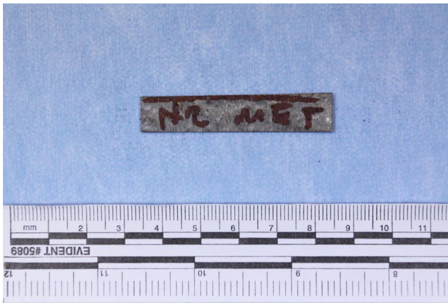
Figure 18. Macro of sample of both sides of hot rolled U-10Mo foil from exterior slice coupon.
