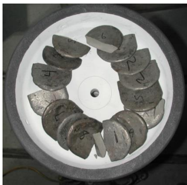
Figure 2. Arc-melted button charge in crucible for U-10Mo casting.
