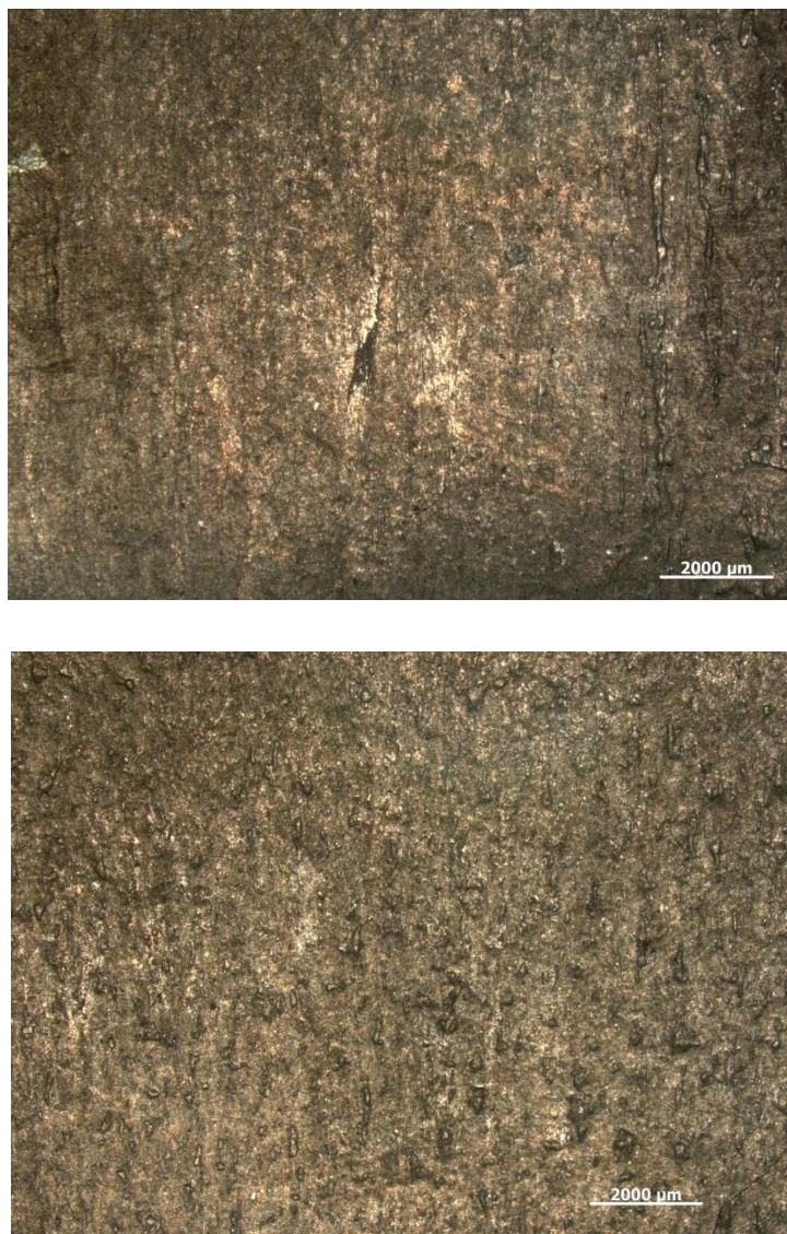
Figure 26. Front and back surface of cold rolled exterior slice U-10Mo coupon. Zr cladding peeled from surface after hot rolling following removal of mild steel can.
