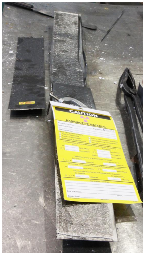
Figure 16. Left: interior coupon following hot rolling with mild steel can removed. Right: Close up of hot rolled interior slice Zr-clad U-10Mo.
