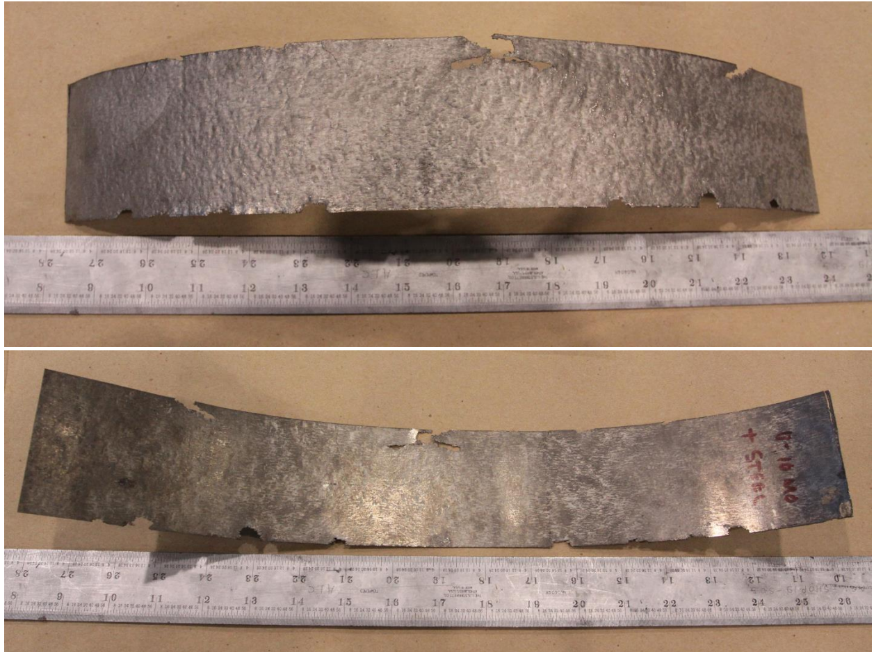
Figure 22. Front and back surface of cold rolled exterior slice U-10Mo coupon. Most of Zr cladding peeled from surface upon steel can removal.
