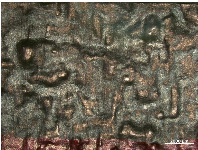
Figure 19. Front and back sides of hot rolled interior slice Zr-clad U-10Mo coupon showing surface roughness.
