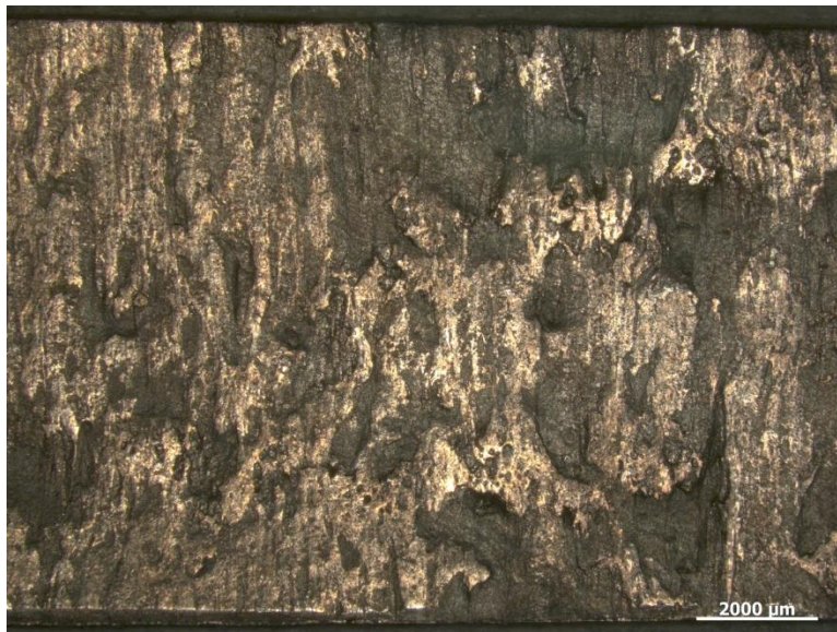
Figure 20. Front and back sides of hot rolled exterior slice U-10Mo coupon showing surface roughness. Most of the Zr cladding adhered to the steel can.
