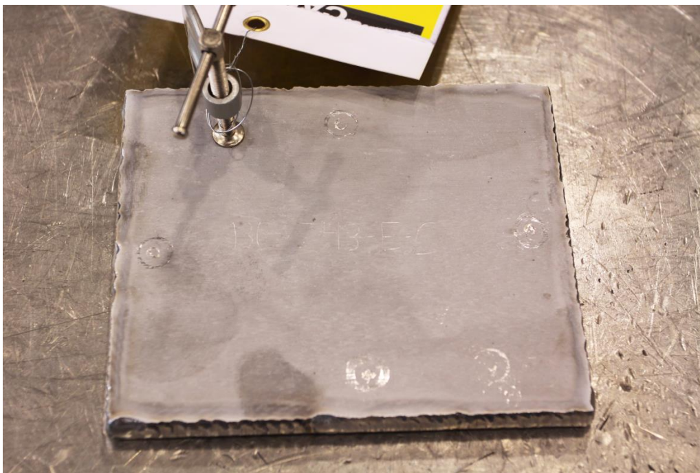
Figure 15. Welded mild steel can for interior U-10Mo coupon.
