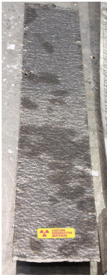
Figure 16. Left: interior coupon following hot rolling with mild steel can removed. Right: Close up of hot rolled interior slice Zr-clad U-10Mo.
