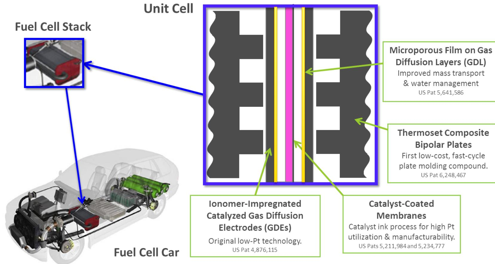
*LANL's innovation in fuel cells technology has played a critical role in the technical viability of fuel cell stacks for FCEVs*
