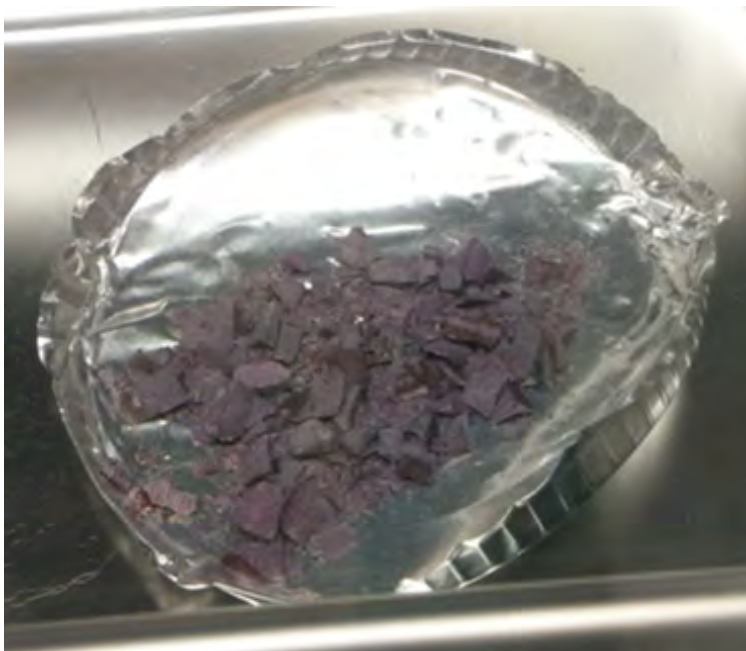
Figure 6.2: Picture of the crushed UCl 3 -LiCl-KCl salt prior to being loaded into the nebulizer.
