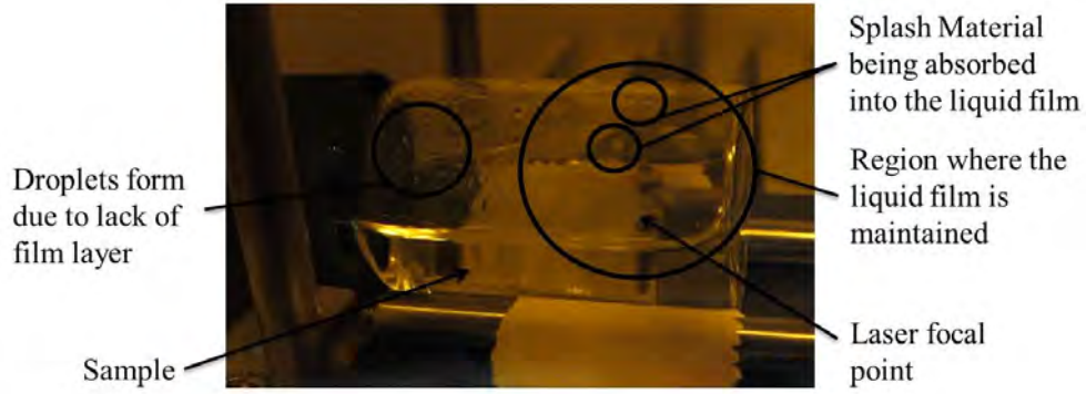
Figure 3.3: Photo of a test vial containing the various splashing and film regions.
