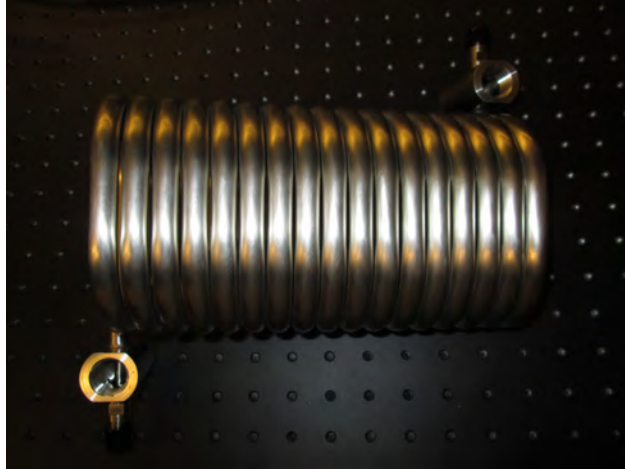
Figure 4.7: Photo of the tube in tube heat exchanger.
