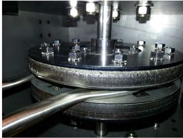
Figure A.4: Close up of the disc positioned around the molten salt loop channel.
