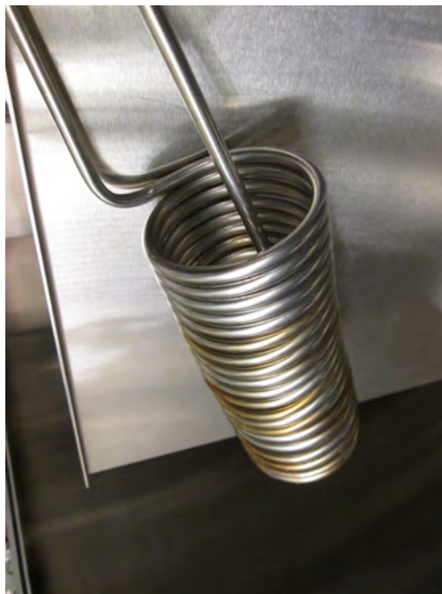
Figure 4.3: Picture of the heating coil manufactured in-house.
