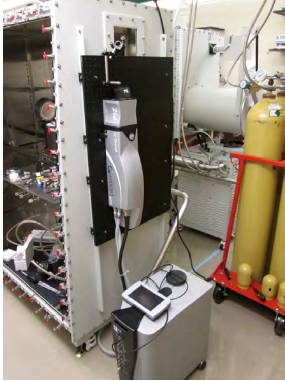
Figure 4.10: Picture of the Q-smart laser mounted to the glovebox and optics used to direct the beam through the window and into the glovebox.
