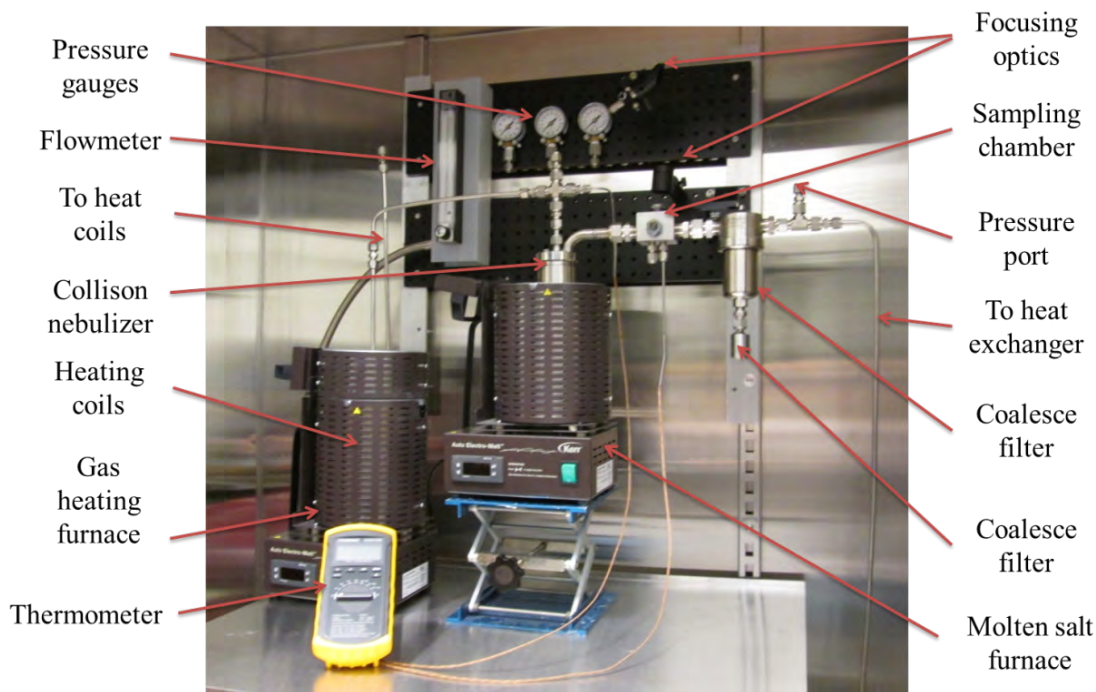
Figure 4.8: Picture of the aerosol system assembly.
