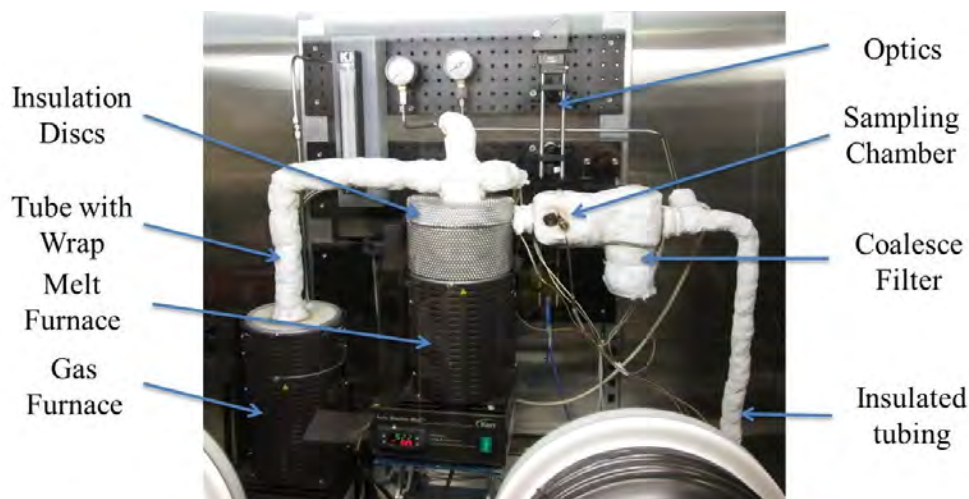
Figure 5.1: Initial high temperature aerosol-LIBS configuration with insulation and heating.
