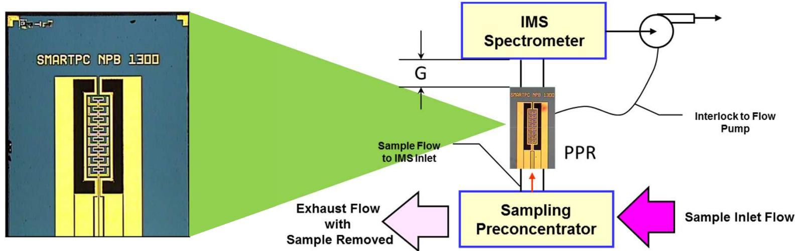
PPR device with paddle width of 500  $\mu\text{m}$  and length of 1500  $\mu\text{m}$
