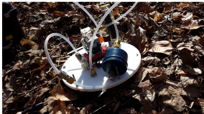
Fig. 1 Field soil collar covered with a Teflon plate equipped with inlet and outlet ports with the former connected to a pump as well as charcoal and ozone filters. All connections were made with Teflon tubing.
