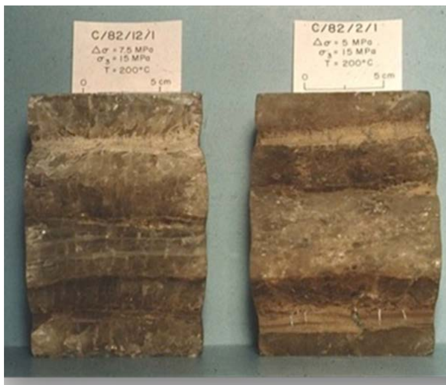
Figure 4-10. Creep tests on bedded salt with anhydrite stringers.
