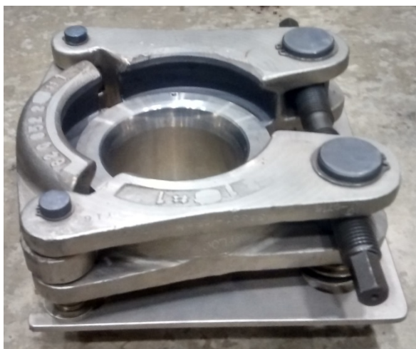
Figure 3-12. Remotely-actuated Grayloc® flange connection system (ORNL photo).
