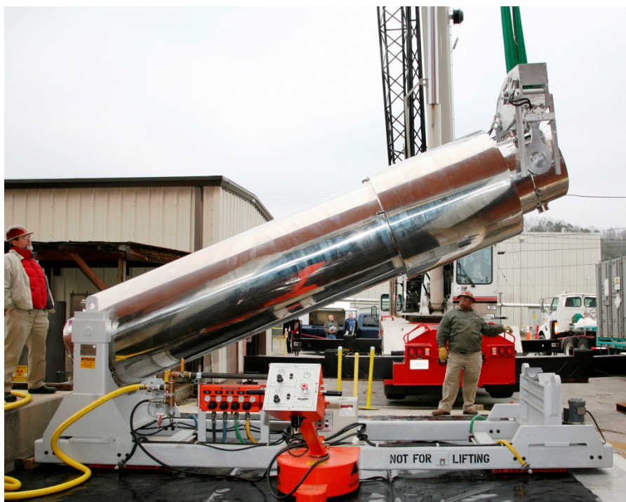
Figure 3-4. LWT cask being lowered into a horizontal cradle (ORNL photo).
