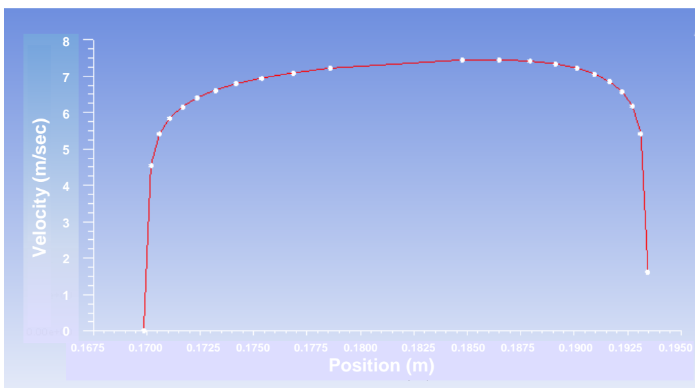
Figure 5-43. Velocity profile (m/sec) in the gap 1 m below the package top.
