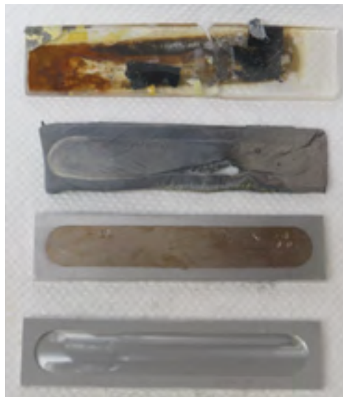
Figure 7. Conditions of the crucible, aluminum target and bismuth before and after distillation.
