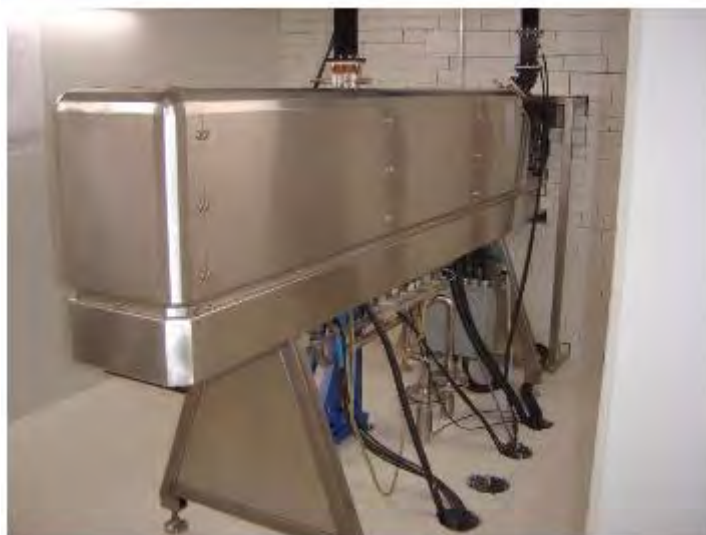
Figure 2.11. MEVEX accelerator used for the production of molybdenum-99. Also, these MEVEX accelerators can come in a clustered accelerator facility which can have up to four accelerators in one facility and is shown below in Figure 2.12 [12].
