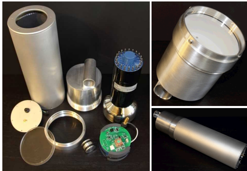
Figure 3. Detector cell components (left), assembled liquid scintillator cell (top right), and complete detector assembly (bottom right).
