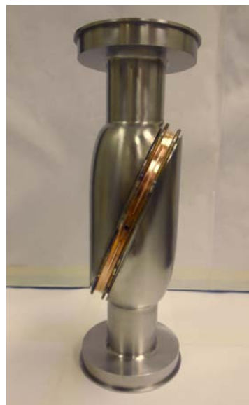
Figure 22. Diamond Brewster angle window vacuum envelope prior to installation of water cooling jacket
