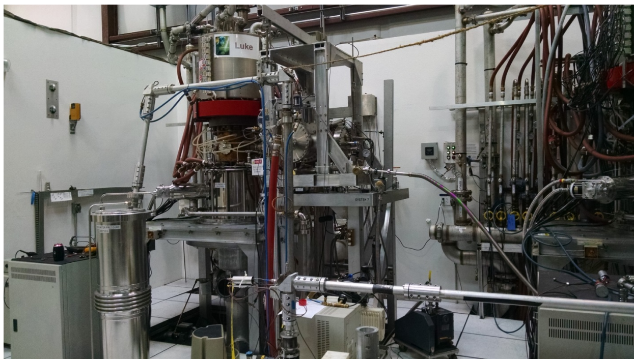
Figure 28. “Luke” 1 MW 110 GHz gyrotron used in the tests at GA.
