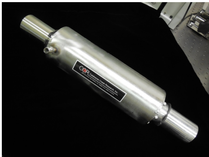
Figure 23. Fully assembled CVD diamond Brewster angle window
