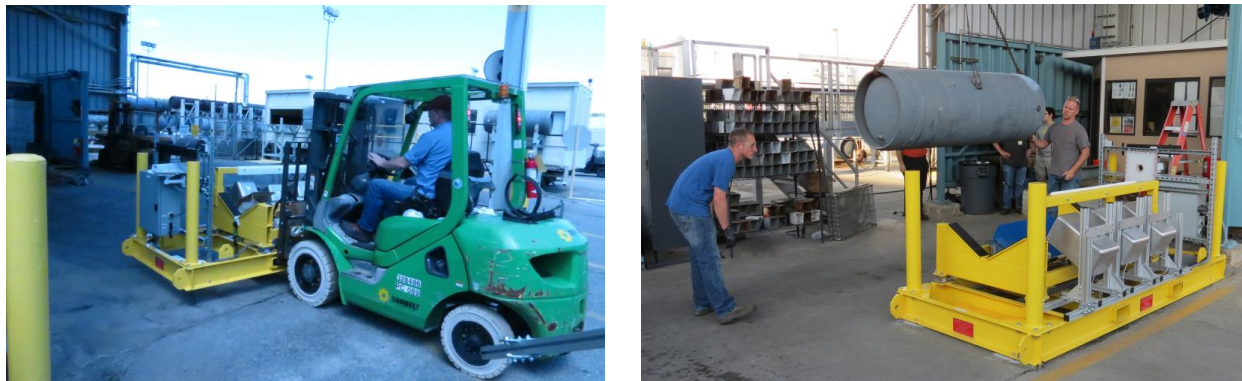
Figure 37. Forklift placement of the platform at the deployment location (left); placement of first cylinder on the UCVS prototype platform using the overhead crane (right).
