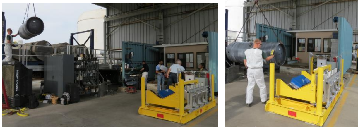
Figure 39. Retrieve a full cylinder from overpack (or other on-site location) and place cylinder on the UCVS platform using the overhead crane. For a typical cylinder scan, the valve/nameplate end of the cylinder should be facing the scale shack.
