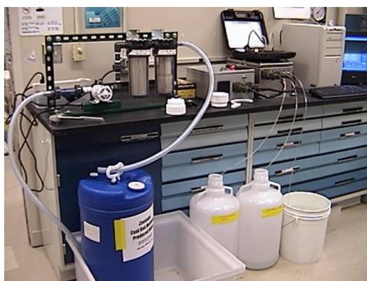
Figure 2-11. A lab-scale configuration for performance testing of Capacitive Deionization technology.
