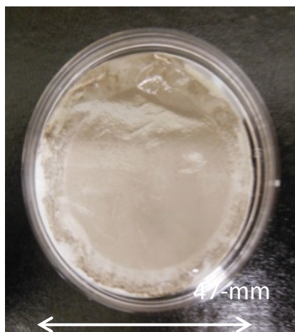
Figure 8-2. Sandia developed graphene oxide (GO)/polymer membrane.
