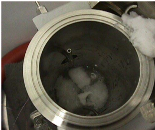
Figure 3-7. Ethylene hydrates formed at 5°C and 370 psi.
