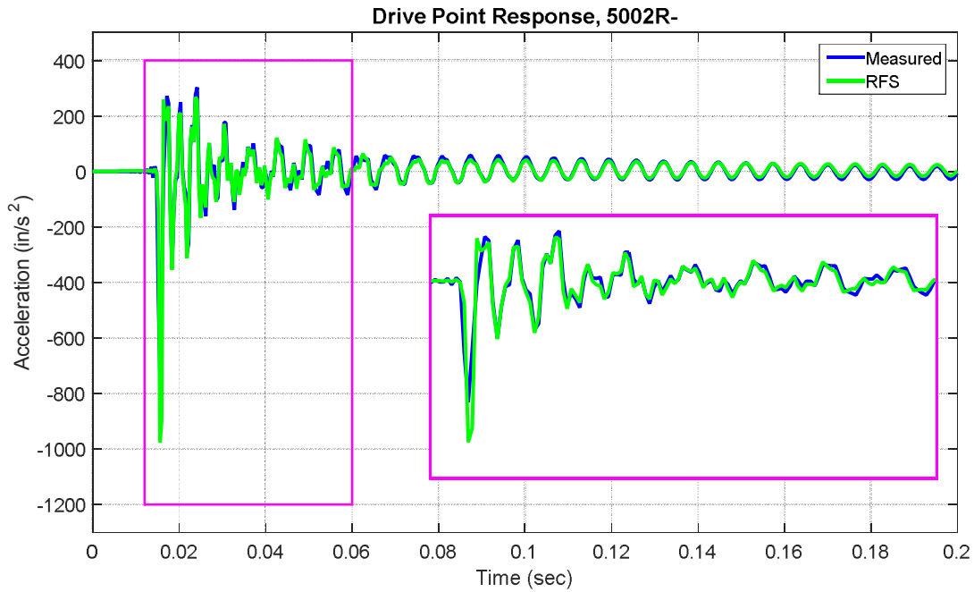
Figure 17 - Radial drive point response, RFS versus measured
