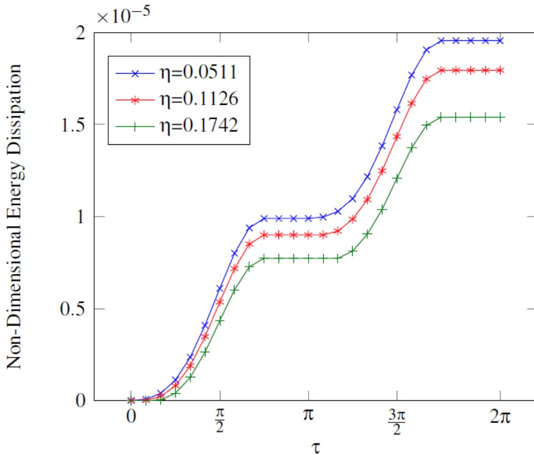
Energy dissipated over a cycle shows expected flat spotting.
