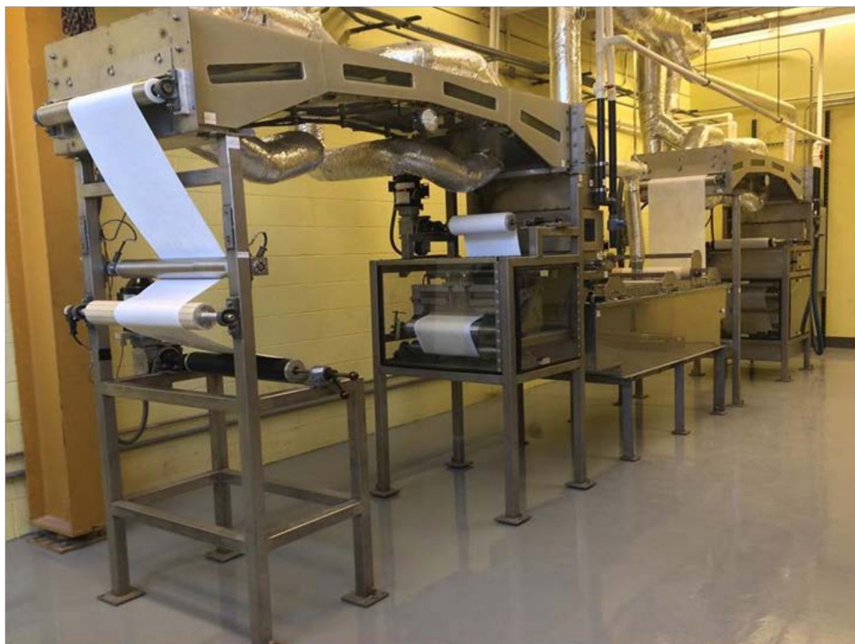
Fig. 10. The continuous membrane coating machine with thin-film casting assembly at OSU.
