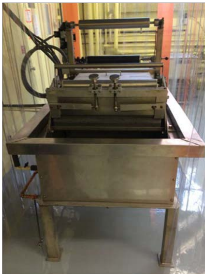
Fig. 12. The continuous casting machine for the fabrication of nanoporous polymer supports at OSU (with fume hood curtains open to show the casting trough and knife).
