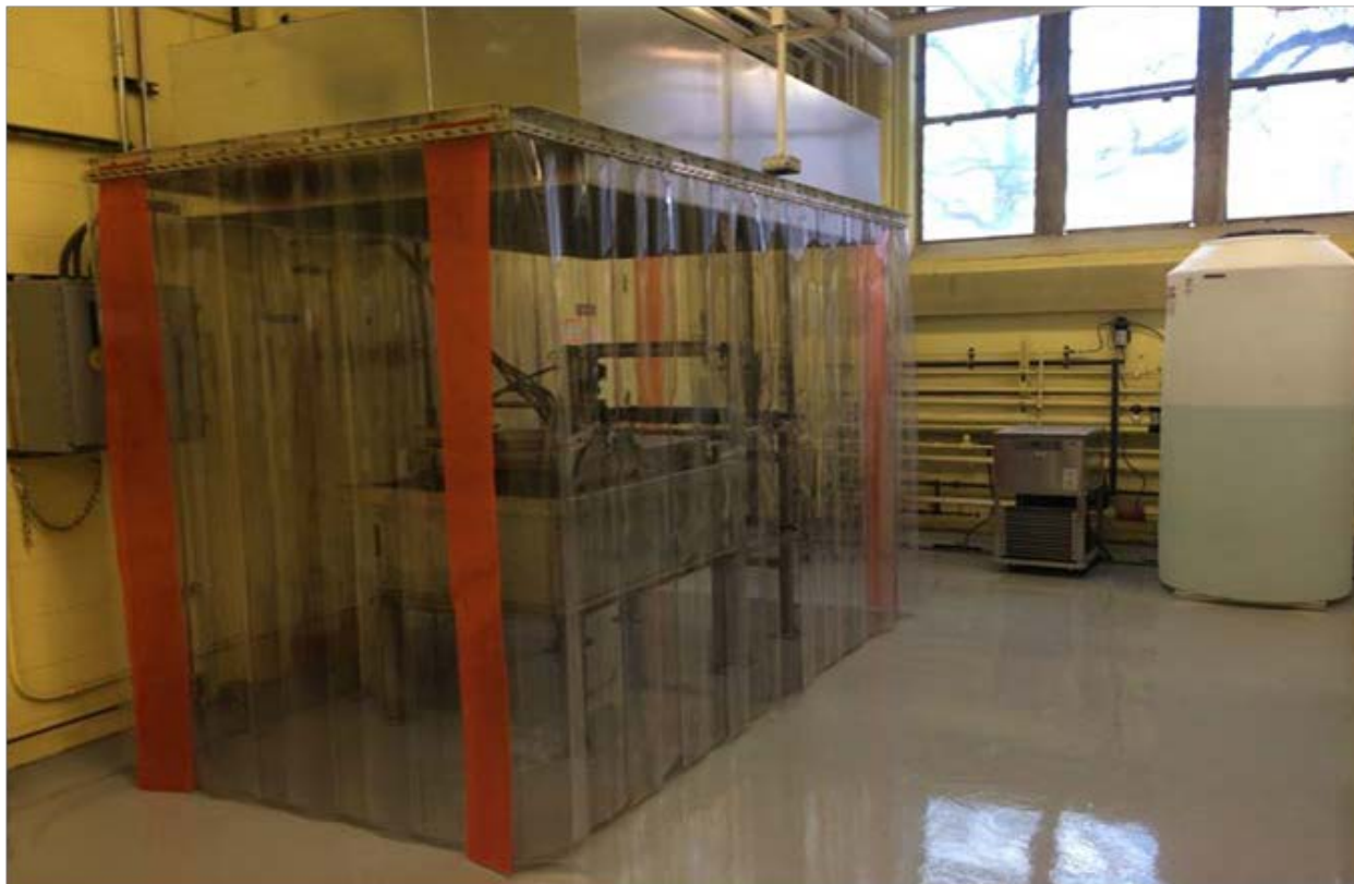
Fig. 11. The continuous casting machine for the fabrication of nanoporous polymer supports at OSU.
