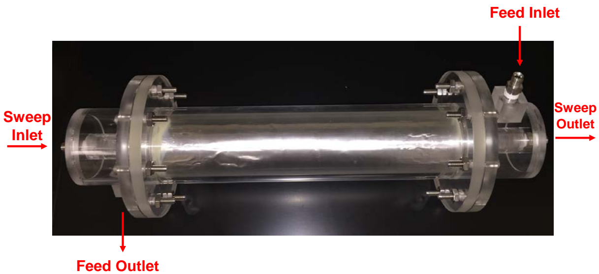
Fig. 16. Spiral-wound membrane module consisting of the membrane element inside a housing.
