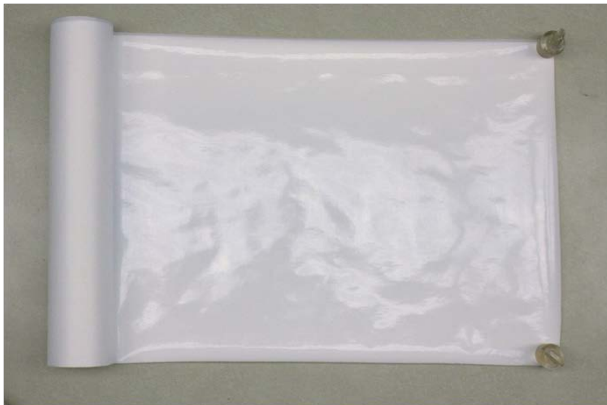
Fig. 13. PES fabricated using the continuous casting machine.
