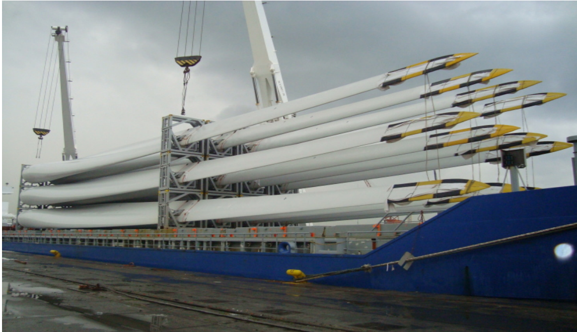
Figure 3-7: Modular Support Frames Used for Stacking and Sea-Fastening of Turbine Blades
