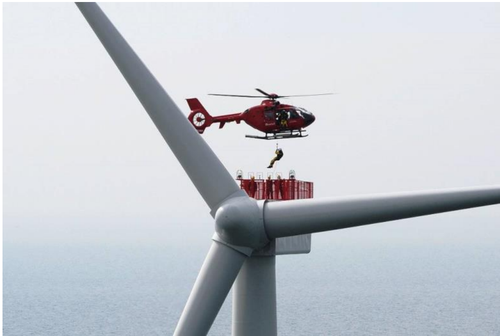
Figure 4-21: Helicopter Hoisting Operation
