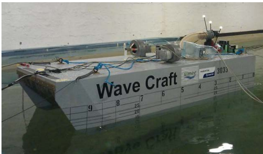
Figure 4-34: Tank Testing of a Model of the Surface Effect Ship
