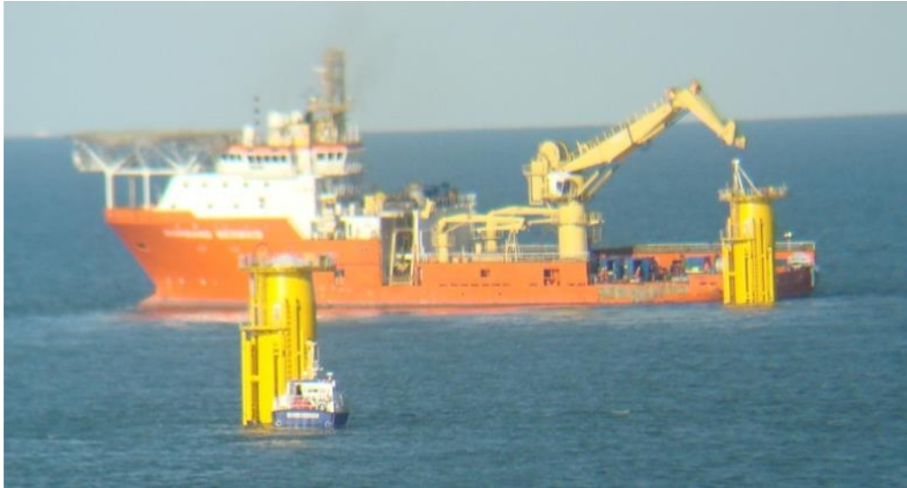
Figure 3-26: Normand Mermaid DP Vessel Used for Array Cable Laying at the Thanet Project, UK
