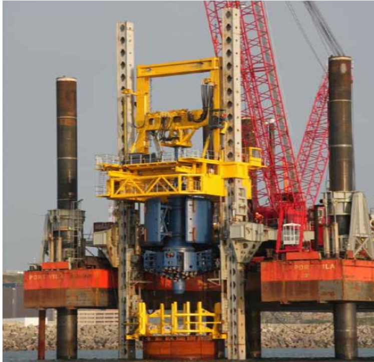
Figure 3-13: Fugro Seacore Toledo 90, Mounted on Jack-Up Vessel Excalibur
