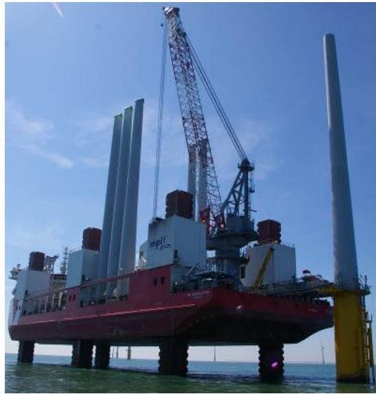
Figure 4-51: MPI Resolution 6-leg, Self-propelled Jack-up
