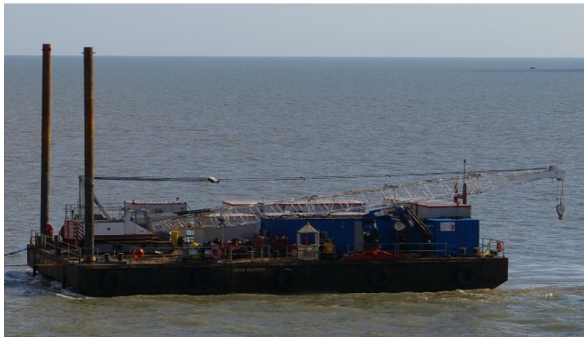
Figure 3-48: Deck Barge with Spud-Legs, and Crawler Crane
