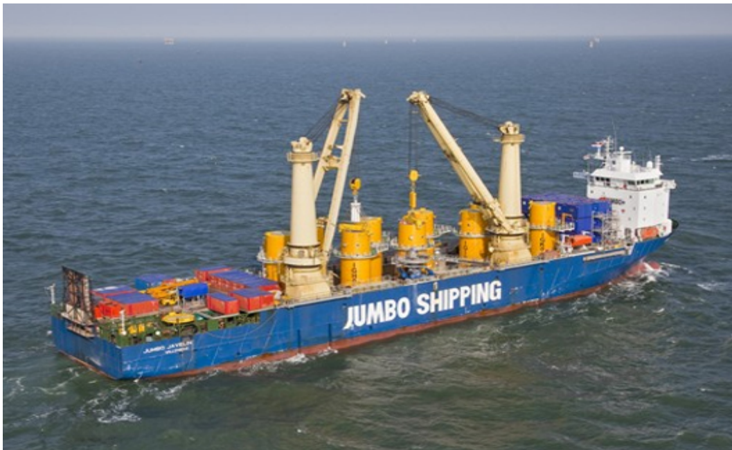
Figure 3-5: Pedestal Cranes on Jumbo Shipping's Jumbo Javelin Used to Install Transition Pieces at the Greater Gabbard Offshore Project
