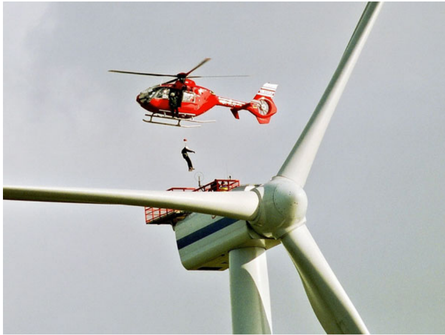
Figure 4-20: Helicopter Hoisting Operation at Horns Rev Offshore Wind Project
