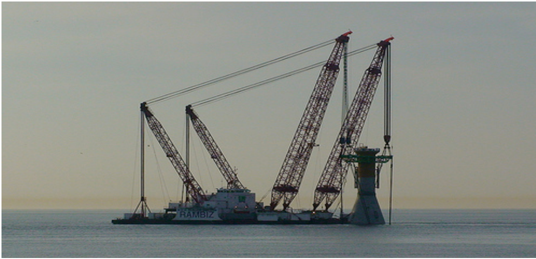
Figure 3-23: Scaldis Rambiz Sheerleg Vessel Transporting a Partially Submerged GBS to Thornton Bank Offshore Project in Belgium
