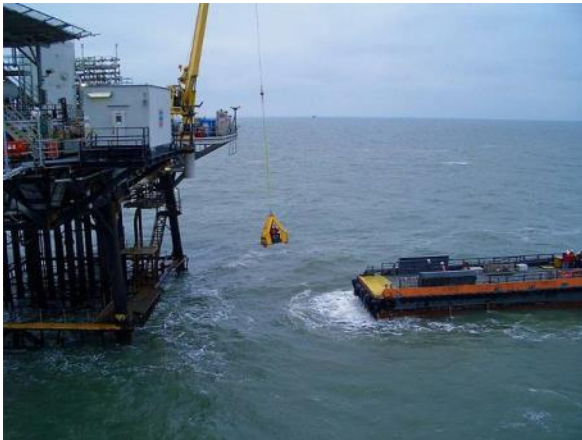
Figure 4-38: Reflex Marine, FROG-3 Crane Transfer Trials on Main Pass 41 in the Gulf of Mexico
