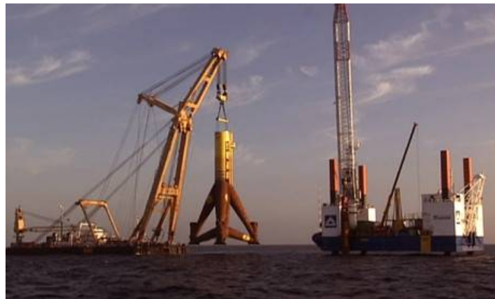
Figure 3-49: Sheerleg Crane Vessel Taklift 4 Working in Tandem with a Jack-up Piling Vessel
