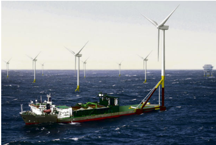
Figure 3-47: SPT Offshore Self-installing Wind Turbine, Tribucket Foundation Concept
