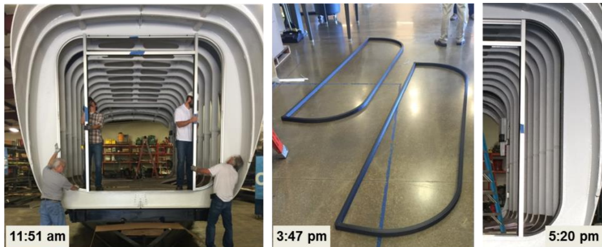
Figure 14. Replacement of over-sized end wall frames using 3D printed sections.
